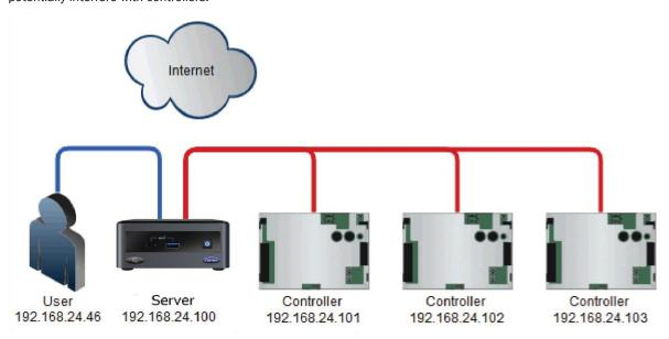
In this example, each controller's BACnet firewall should allow BACnet communication from the i-Vu® Express server's IP address and the controller's IP addresses. The user at 192.168.24.46 should not be allowed BACnet communication with the controllers.
