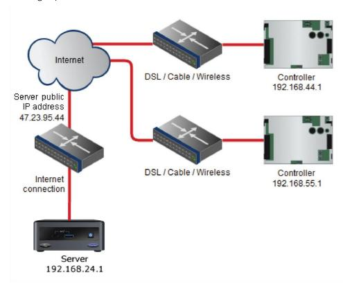
In this example, each controller needs to communicate with only the i-Vu® Express server so their BACnet firewall's whitelist should have only the server's public IP address. The controllers do not need to communicate with each other.
