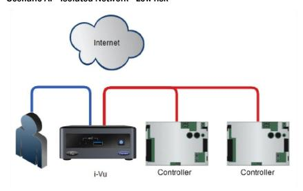
Do not permanently expose the i-Vu Express server or the BACnet network to the Internet. You can, however, allow users to access the i-Vu Express server through a secure VPN connection. If a NAT router or firewall is present on the LAN for other purposes, it should not have any ports forwarded to the i-Vu Express server or any controllers.
