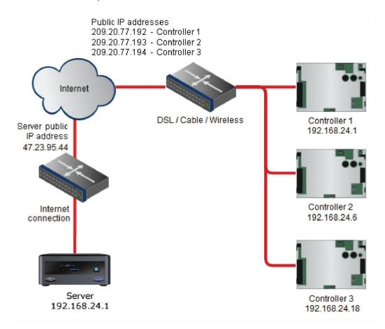
In this example, the controllers need to communicate with the i-Vu® Express server and each other. The controllers are the only devices on the site's private network, or other devices present are benign.
