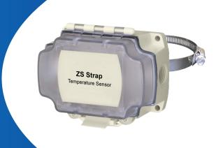
The Carrier communicating ZS clamp-on strap sensor is designed to monitor water temperature in retrofit or filled pipe applications. This sensor has a bendable copper sensing plate that forms to the curvature of the pipe, along with an adjustable hose clamp that holds the unit in place around the pipe. It measures the water temperature by sensing the surface temperature of the pipe.
