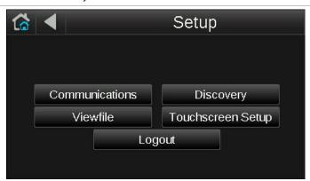
Touch a button to go to the **Communications**, **Discovery**, **Viewfile**, or **Touchscreen Setup** screen, or to log out.
