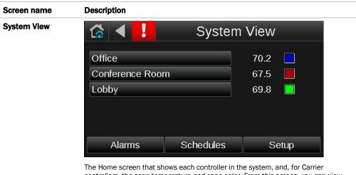
The Home screen that shows each controller in the system, and, for Carrier controllers, the zone temperature and zone color. From this screen, you can view alarms or set up schedules. A user with an administrator-level password can edit the system or edit touchscreen settings. This screen displays when the System Touch has had no user activity for a period of time specified on the *Touchscreen Setup* > **Inactivity Timeout** screen (page 16).
