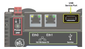
To access the router setup pages and use the **Local Network** tab, you must first connect to and manually address one TV-CRB-E2. For instructions on connecting, see *Addressing the TV-CRB-E2 through the USB Service Port*.(page 6). Navigate to http://local.access or http://169.254.1.1 to access the pages. Then set up the address on your selected TV-CRB-E2 on the **Ports** tab.
