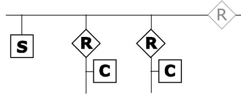
3 BACnet routers separated by an IP router (page 27)
