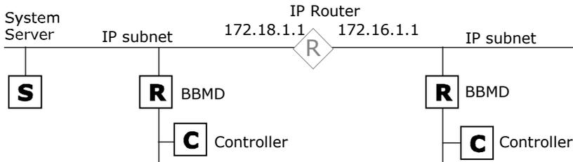
**NOTE** A BACnet SC router cannot be a BBMD device. Ensure that at least one of your downstream BACnet IP devices is the assigned BBMD, and is on the same subnet and the Gig E port connection for the BACnet SC router.
