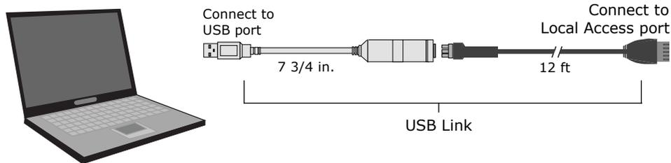
**NOTE** If using a USB isolator, plug the isolator into your computer's USB port, and then plug the USB Link cable into the isolator.
