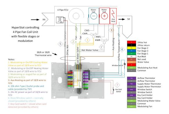
For 4-pipe FCUs, select the 4-pipe FCU profile to obtain the required sequence:
