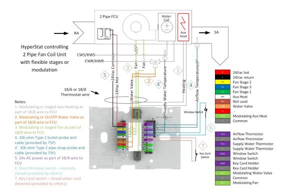
For 2-pipe FCUs, unit ventilators, and induction units select the 2-pipe FCU profile to obtain the required sequence:
