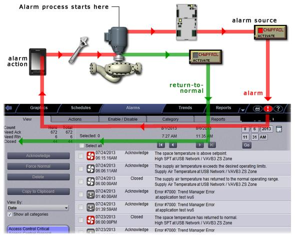
Alarm sources and the alarms they generate are assigned to categories, such as HVAC Critical or HVAC Maintenance, to help you work with related alarms.
