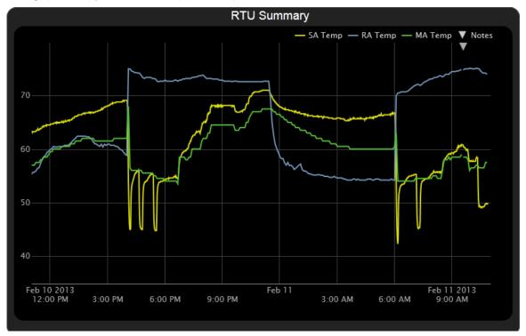
You can collect trend data for any point value in the i-Vu® system. The controller reads point values at intervals that you define and then stores that data in the controller for up to 7 days. A controller has limited memory for storing trend data, so you can set up historical trending to archive the trend data from the controller to the database.
