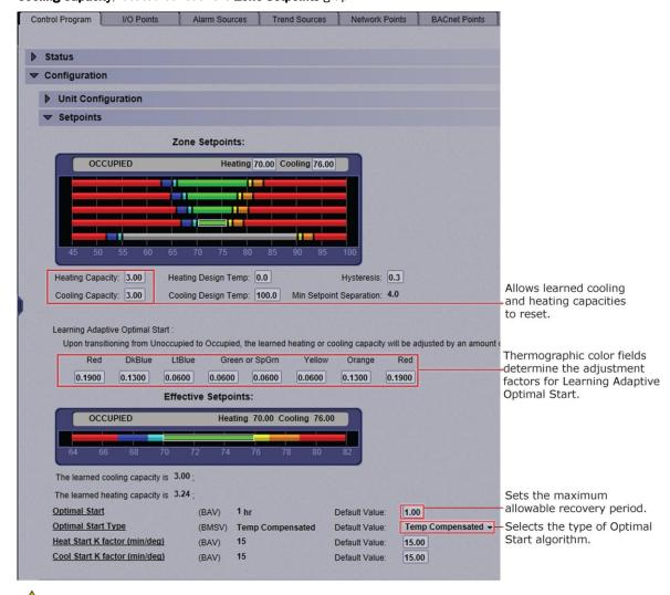
**CAUTION** When using **Learning Adaptive Optimal Start**, be sure that all equipment is properly maintained so that your system does not "learn" to compensate for dirty filters or loose fan belts.
