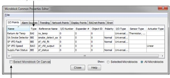
Select this checkbox and then select a point in the list to locate that microblock in the control program.
