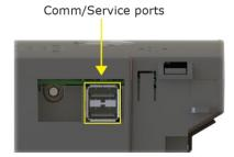
**CAUTION** The USB local access cable provides a common ground connection between the computer and the controller it connects to. Damage to the controller and possibly the computer's USB port will occur if the controller's input power polarity was not maintained and was also not properly grounded (floating). If you are not sure of the wiring polarity and that the controller was properly grounded, use a USB isolator between the computer and the controller.
