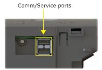
To access the controller setup pages and use the **Local Network** tab, you must first connect to and manually address one TV-VVTBP-E2. For instructions on connecting, see *Addressing the TV-VVTBP-E2 through the Comm/Service ports* (page 15). Navigate to http://local.access or http://169.254.1.1 to access the pages. Then set up the address on your selected TV-VVTBP-E2 on the **Ports** *tab* (page 58).
