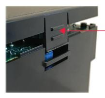
Press tab and pull up to open and remove cover
