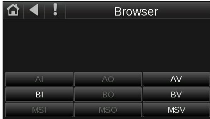
Touch a button to see that type of BACnet objects found in the controller. Each screen shows a list of network-visible BACnet objects with BACnet Object Name, Current Value, and BACnet Object Instance number.
