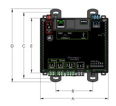
Controller (part no. TV-022-E2) Installation and Start-Up Guide Carrier Proprietary and Confidential
