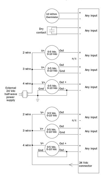
4 Connect binary and analog output wiring to the screw terminals on the TV-VVTZC-E2 and to the controlled device.
