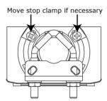
**9** Hold down the actuator release button, rotate the damper to verify that it opens and closes, then release the button.
