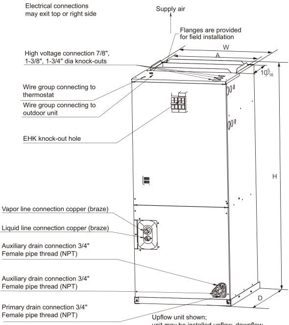
unit may be installed upflow, downflow, horizontal right or left air supply.
