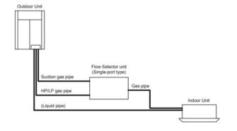
The single port flow selector box does not have a liquid refrigerant piping connection. Liquid refrigerant piping should connect directly to the indoor unit when using the single port flow selector box
