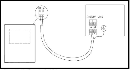
Use wire size 18AWG stranded, shielded, 2-core
