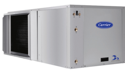
Aquazone™ 50PSH, PSV Horizontal/Vertical Upflow 0.5 to 6 Tons R-410A Exceeds ASHRAE 90.1, AHRI Certified
