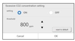
Settings of CO<sub>2</sub> concentration excess and threshold can be set. If the setting is enabled, Check Code S36 is generated when the CO<sub>2</sub> concentration exceeds the threshold.
