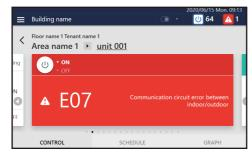
• If a malfunction occurs, a check code is displayed. Operation other than operation ON/OFF is not possible.
