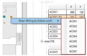
If you draw wiring for an FS unit to an indoor unit icon with a different indoor unit name, then it is shown as a dotted line.
