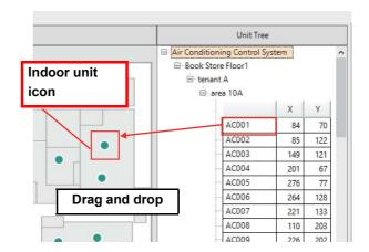
The figure on the right shows an example of the coordinates when placing an indoor unit icon.
