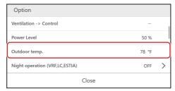
You can check the outdoor temperature detected by the outdoor unit.
