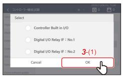
2 Select a digital input/output interface or I/O built-in to the main unit.
