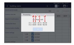
Acquisition of DN setting values from outdoor units is in progress. The states of the settings for the DN setting values are shown.
