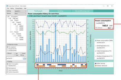
For [Power Consumption], both the graph total value and  ${\rm CO_2}$  emissions are shown to one decimal place when they are less than 1000.
