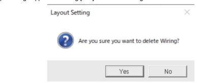
If you have drawn multiple wires to an FS unit icon, you can also select from the menu and delete indoor unit icons to which the wiring is connected.
