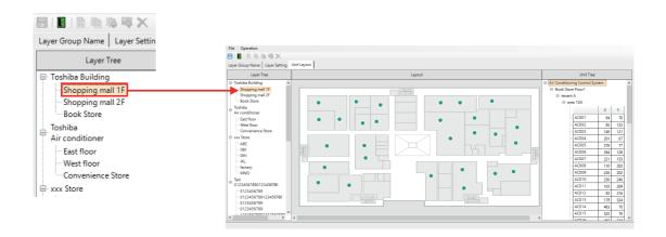
Enter the "X coordinate (horizontal)" and "Y coordinate (vertical)" for the indoor unit you want to place from the "Unit Tree" view. Alternatively, you can drag and drop the indoor unit onto the layer layout.
