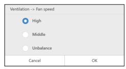
You can set the ventilation fan speed of the ventilator connected to the air to air heat exchange unit or the air conditioner. The choices displayed depend on the model.
