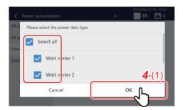
**4** To select [3-(3)] or [3-(4)], set the check box of the watt hour meter to sum to **✓** and tap [4-(1)]
