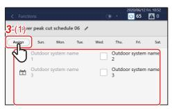
3 Tap [3-(1)] and set the check box of the outdoor unit for setting the Power peak cut schedule to ✓
