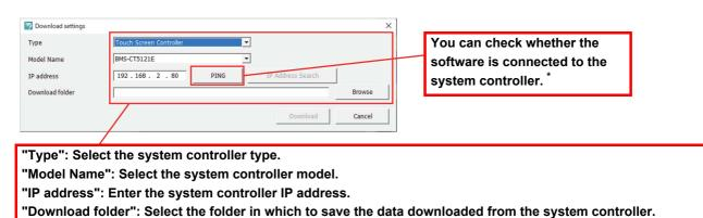
\* Connection check result The images below are examples of the dialogue boxes that appear when checking connection with the system controller.
