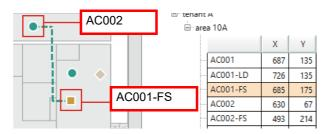
If you change the position of an icon after drawing wiring to that icon, the wiring does not move.
