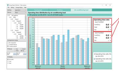
The operating time ratio for operating modes is shown for the selected time period. "Cool" The total value of the operating time ratio of <Cool>, <Dry> and <Auto Cool>.
