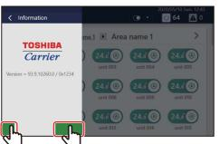
Tap and hold the lower left and lower right of the Information screen at the same time for about five seconds
