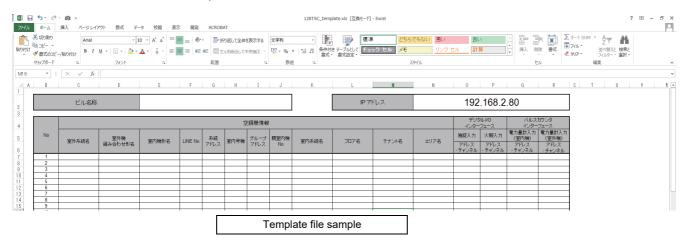
(3)Start up the Setting File Creation Software 2. Select [Tools] - [Import] - [Touch screen controller] - [BMS-CT2560U-UL]\*, and then import the data for the template file.
