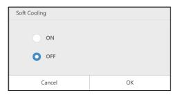
Soft Cooling can be turned ON/OFF. When turned ON, the air direction is set to up, and the maximum power is restricted.
