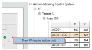
You can select multiple indoor units on the layout screen when you draw wiring to an indoor unit from an FS unit.
