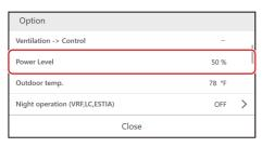
You can check how much power the air conditioner is using for operation.
