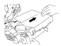
4 Remove the electrical control box cover and set bit1 of SW01 on the board to ON. (Do not touch SW02 as it is used for other setting.)
