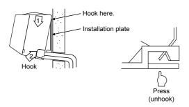
For detaching the indoor unit from the installation plate, pull the indoor unit toward you while pushing its bottom up at the specified parts.
