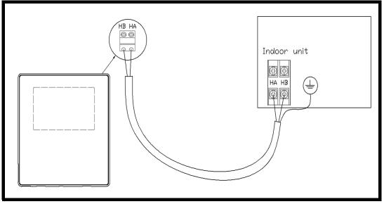
Use wire size 20AWG to 16AWG stranded, shielded, 2-core. ٠
