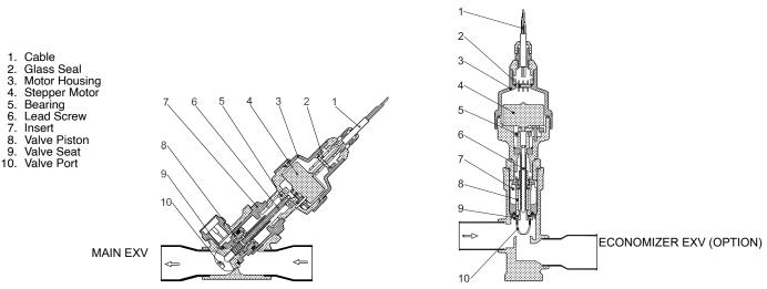
Fig. 21 — Cutaway Views of Electronic Expansion Valves (EXV) (P Compressor Only)
