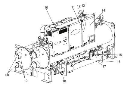
10 — Inductor Temperature Switch (Inside VFD Enclosure)
