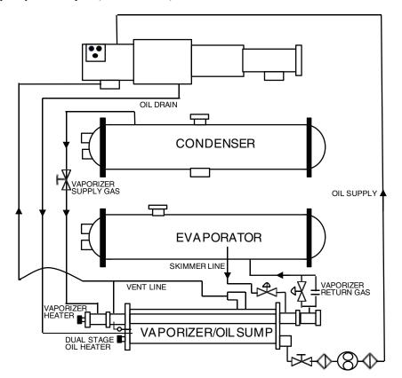
Fig. 13 — Oil Flow Schematic
