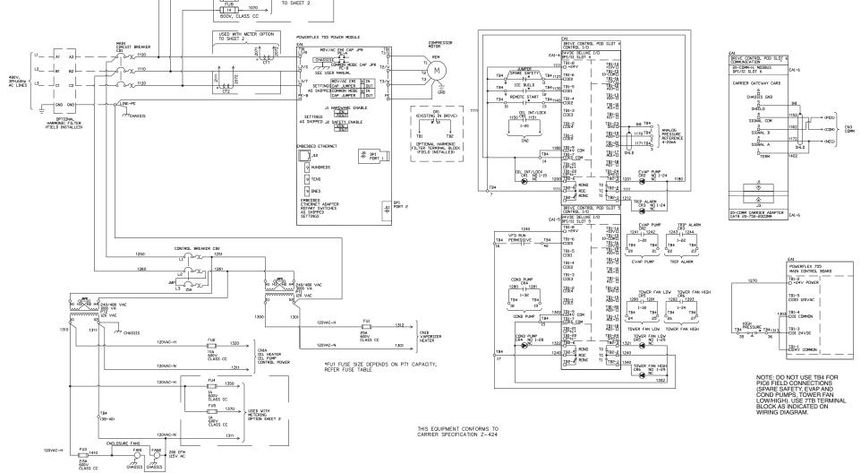
Fig. 64 — 23XRV VFD Schematic (Rockwell Standard Tier VFD)
