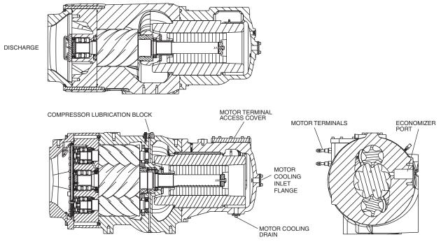
Fig. 8 — Compressor (Typical, R Compressor Shown)
