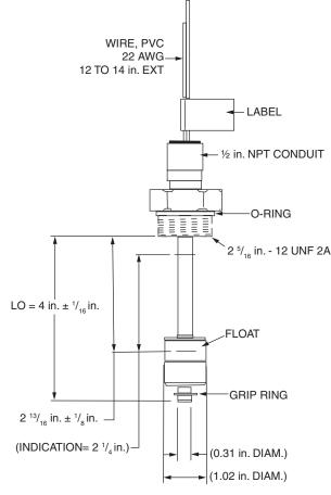
Fig. 61 — Condenser Liquid Level Sensor
