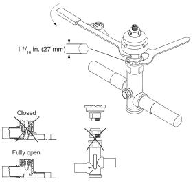
Fig. 58 — EXV Disassembly
