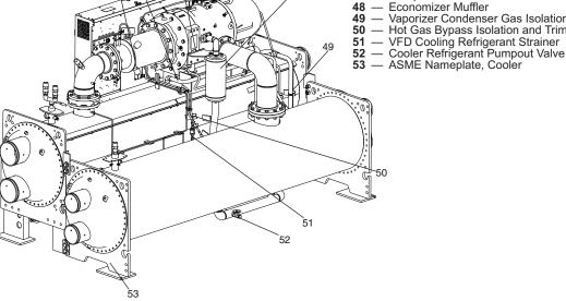
Fig. 3 — Typical 23XRV Components (Units with Q Compressor)
