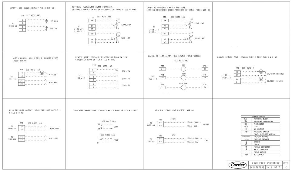
Fig. 62 — 23XRV Controls Schematic (cont)
