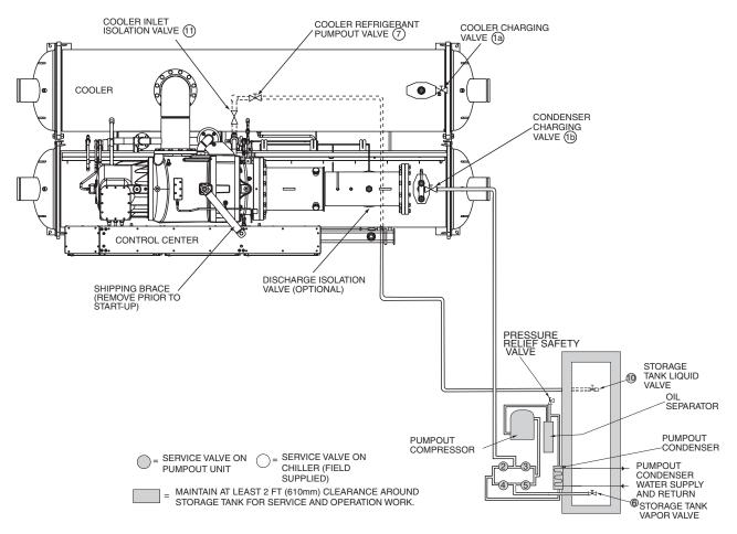
Fig. 28 — Optional Pumpout System Piping Schematic with Storage Tank — Configured to Push Liquid into Storage Tank (Unit with R Compressor Shown)
