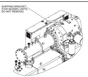
Fig. 45 — Control Center Shipping Bracket (Unit with R Compressor Shown)
