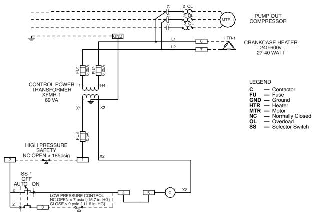
Fig. 48 — 23XRV Pumpout Unit Wiring Schematic
