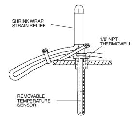
Fig. 14 — Control Sensors (Temperature)
