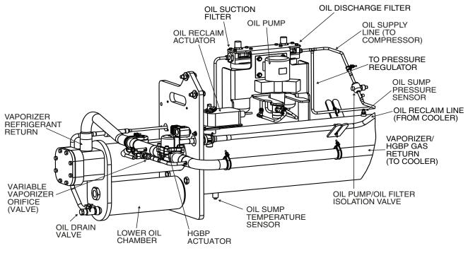
Fig. 52 — 1-Piece Vaporizer Oil Management System
