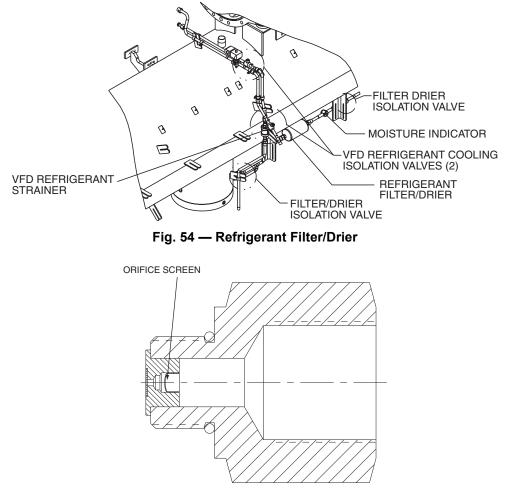
Fig. 55 — Compressor Inlet Bearing Oil Orifice
