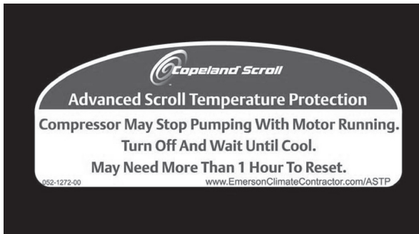
Fig. 24 — Advanced Scroll Temperature Protection Label
