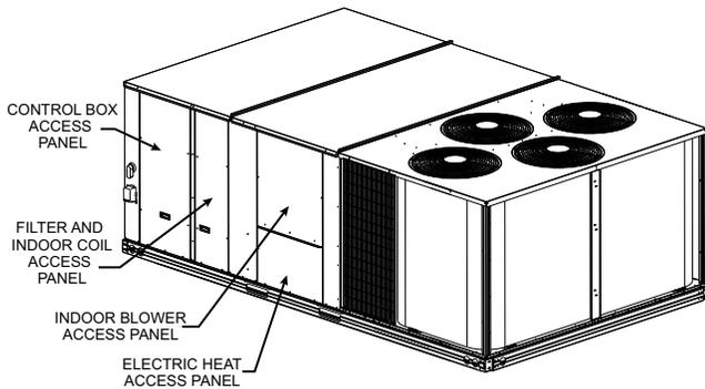
**Fig. 54 — Typical Access Panel Location**
