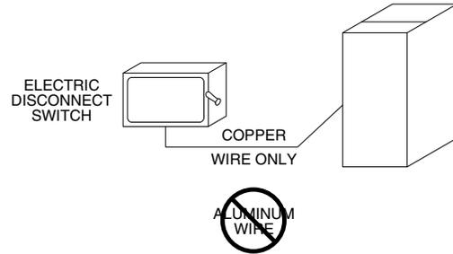
**Fig. 42 — Disconnect Switch and Unit**
