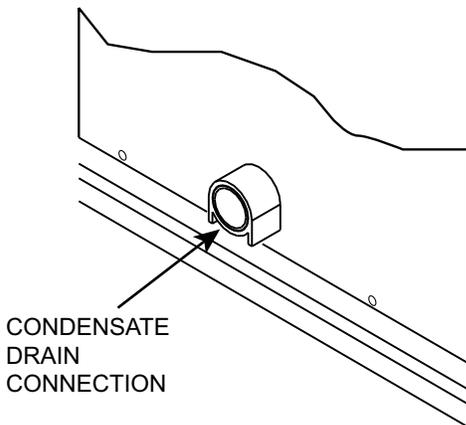
**Fig. 39 — Condensate Drain Pan Connection**
