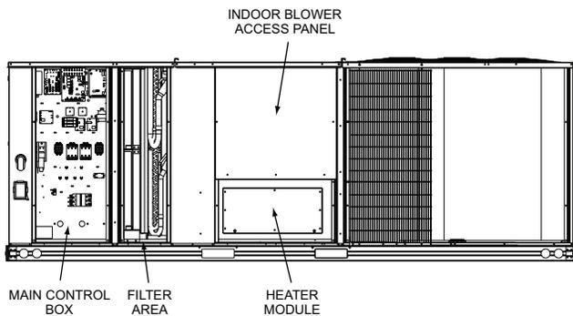
**Fig. 55 — Typical Component Location**
