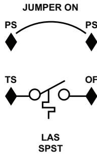
**Fig. 60 — SPST Low Ambient Switch Schematic**
