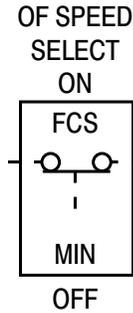
**Fig. 59 — Outdoor Fan Speed Select Switch**
