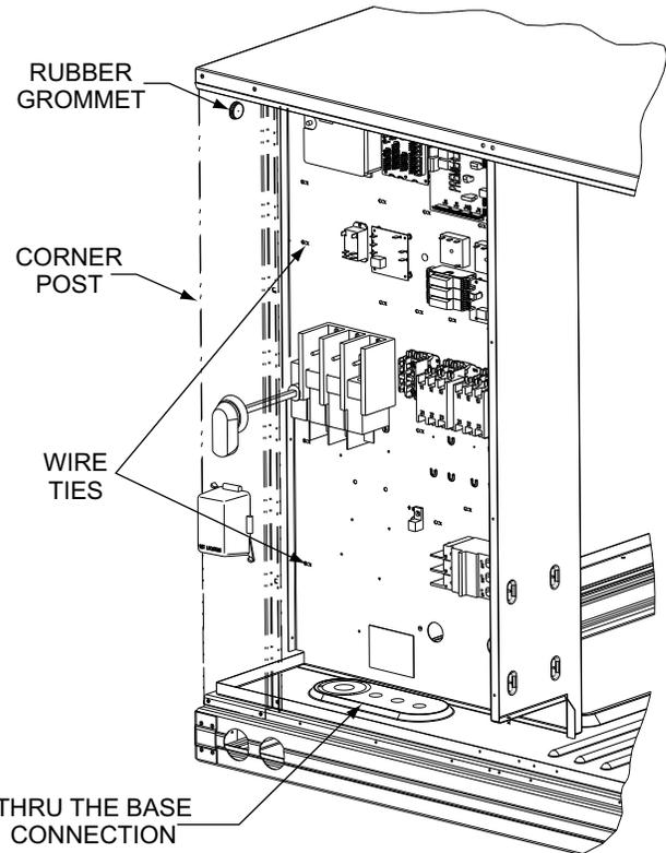
**Fig. 53 — Field Control Wiring Raceway**
