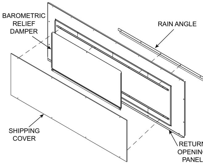
**Fig. 38 — Barometric Relief Damper — Shipping Location**
