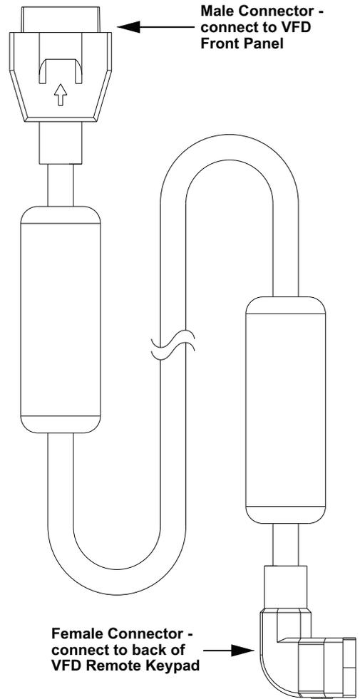
**Fig. 69 — VFD Remote Keypad Cable**
