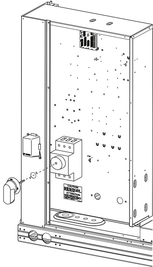
**Fig. 46 — Handle and Shaft Assembly for HACR**
