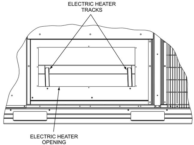
**Fig. 56 — Electric Heater Compartment (Cover Removed)**
