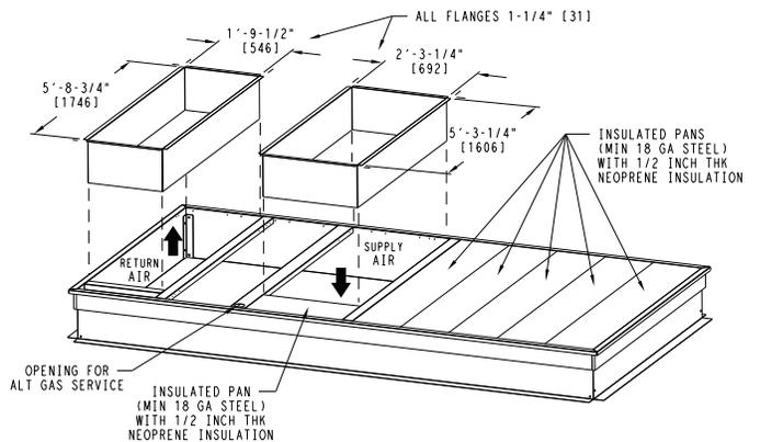
Fig. 21 — Roof Curb Details - 24 and 26 Size Units
