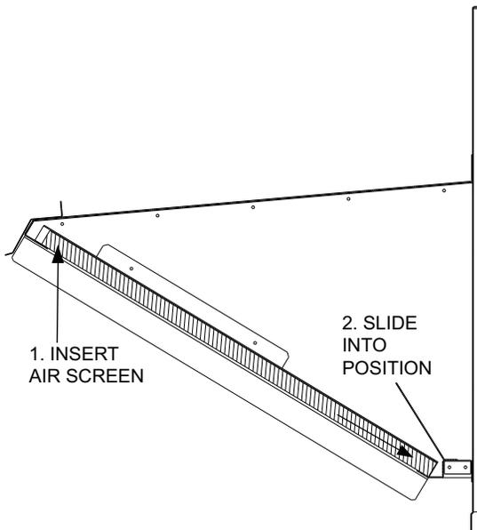
**Fig. 28 — Outdoor Air Screen Installation**
