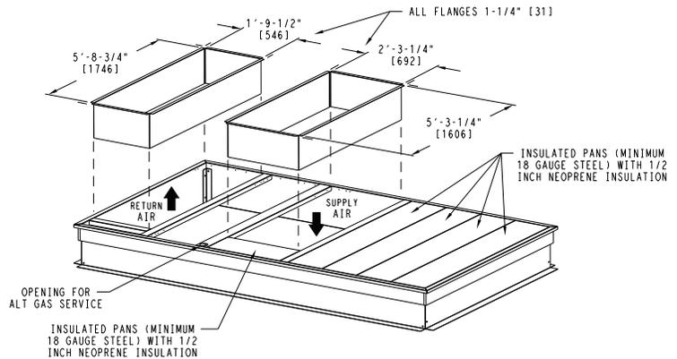
Fig. 20 — Roof Curb Details - 17 and 20 Size Units
