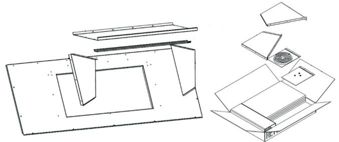
**Fig. 30 — Barometric Hood Parts**
