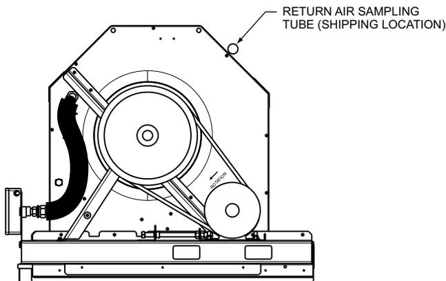
**Fig. 71 — Typical Supply Air Smoke Detector Sensor Location**
