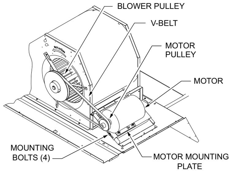
Fig. 75 — Belt Drive Motor Mounting
