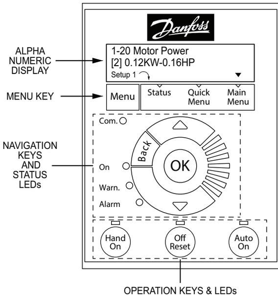
**Fig. 63 — VFD Keypad**
