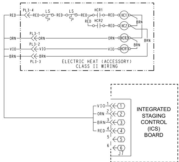
**Fig. 57 — Optional or Accessory Electric Heater Control Connections**
