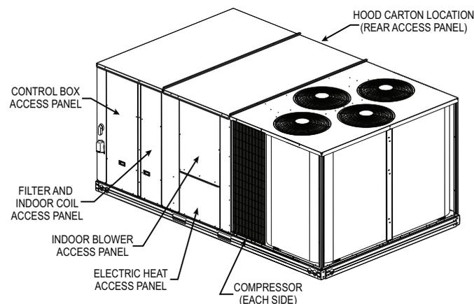
**Fig. 17 — Typical Access Panel and Compressor Locations**
