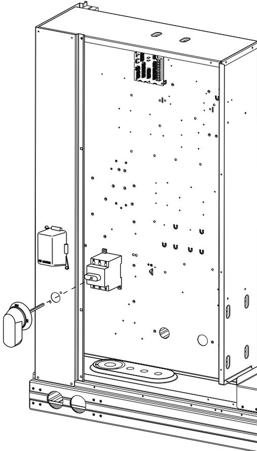
**Fig. 45 — Handle and Shaft Assembly for NFD**
