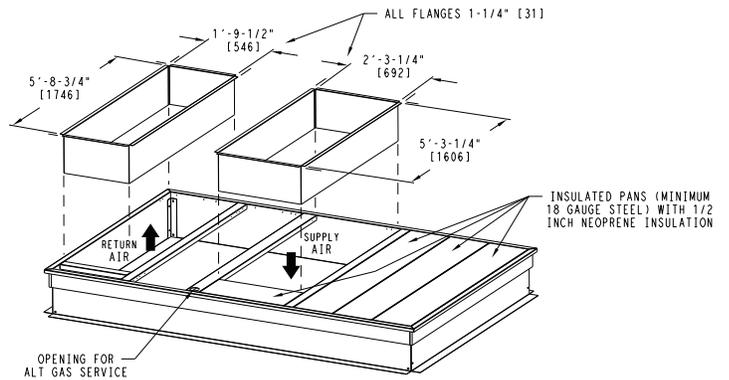
Fig. 19 — Roof Curb Details - 14 Size Unit
