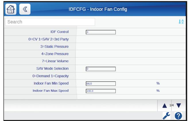
**Fig. 88 — Indoor Fan Configuration Screen**
