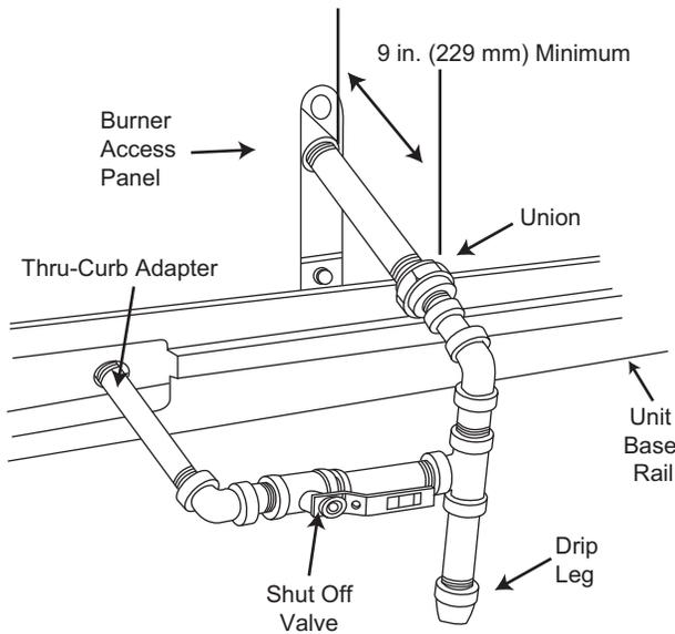
**Fig. 28 — Gas Piping with Offset Drip Leg**
