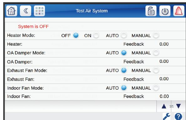
Fig. F — Test Air System Example (Service Run)
