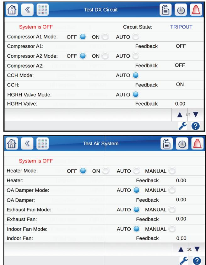
Fig. E — Test DX Circuit and Test Air System Screens (Service Run)
