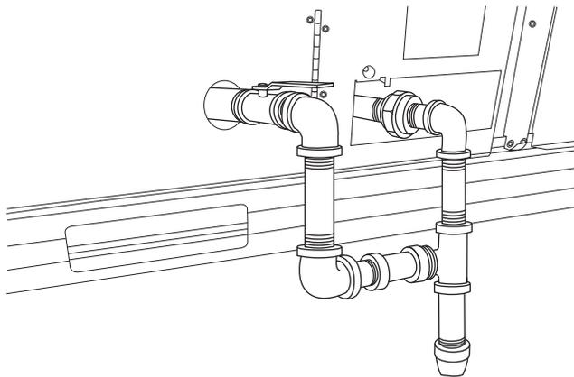
**Fig. 29 — Gas Piping Thru-Base Connections**
