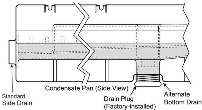
**Fig. 20 — Condensate Drain Pan (Side View)**
