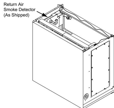
Fig. 56 — Return-Air Smoke Detector (Shipping Position)
