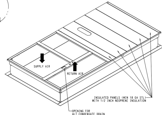
Fig. 7 — Roof Curb Details, Sizes 08-12 Units
