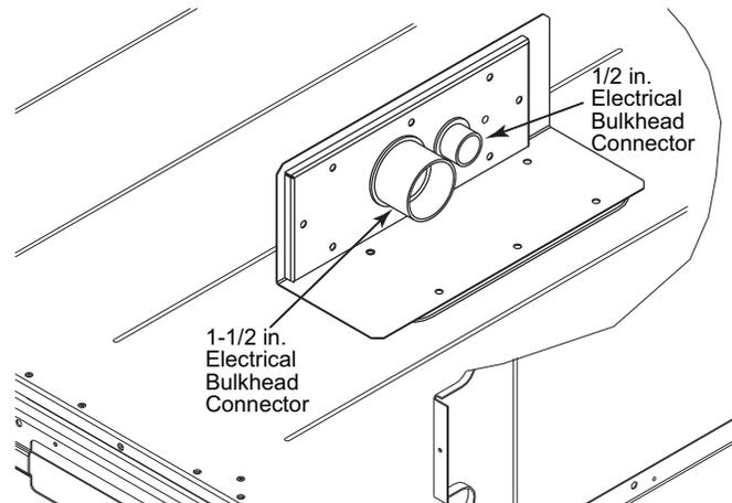
Fig. 52 – Thru-the-Base Option, Shipping Position
