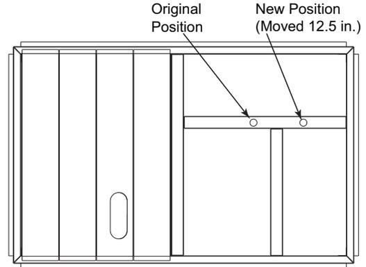
**Fig. 9 — Alternative Condensate Drain Hole Positions**
