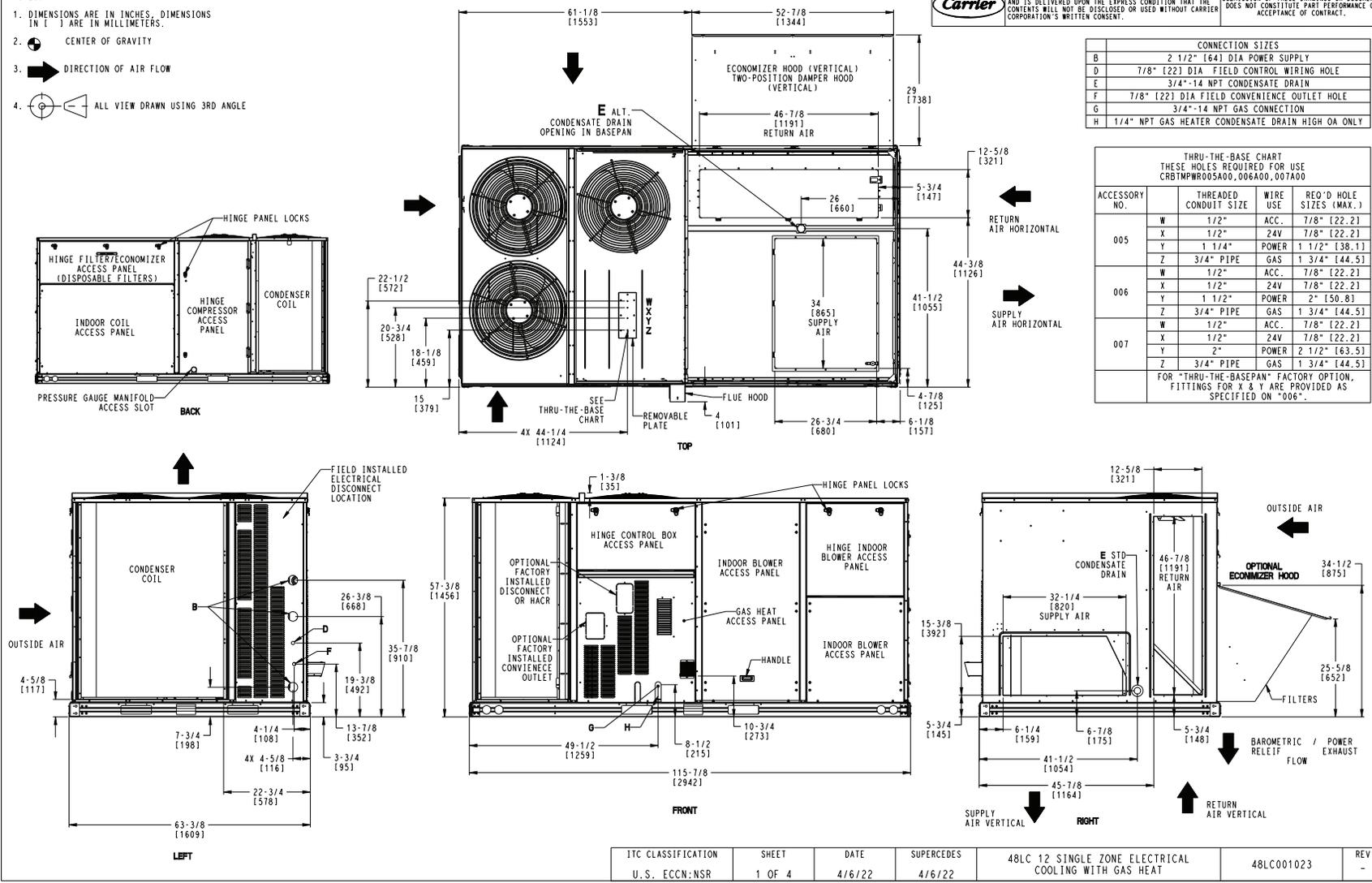
**Fig. 4 – Unit Dimensional Drawing, Size 12, Single-Zone Electric Cooling with Gas Heat**
