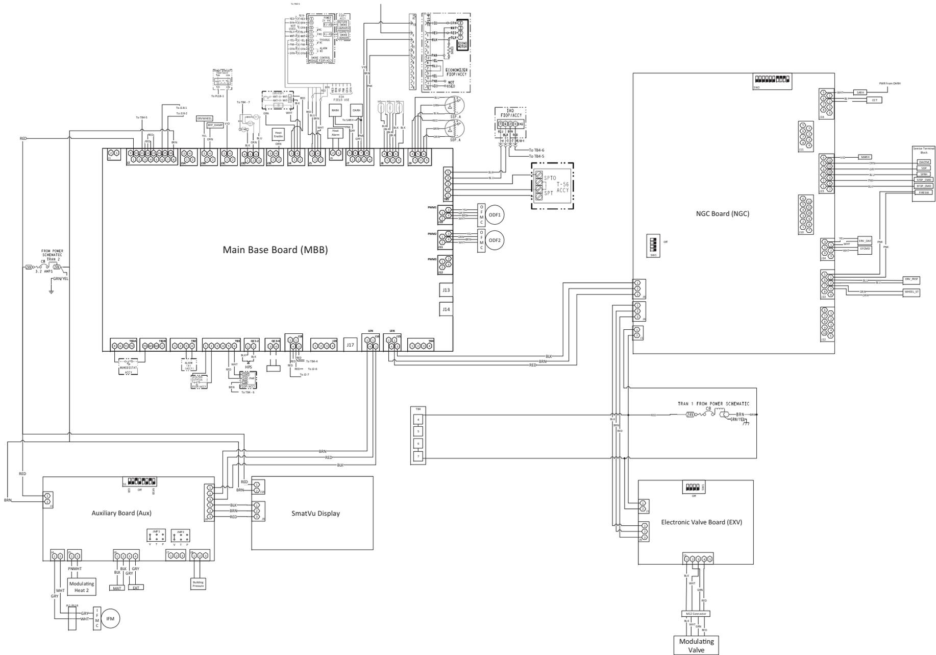
Fig. 36 — 48LC\*H 07 SmartVu™ Control Wiring Diagram (208/230-v, 460-v, 575-v Units)
