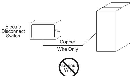
**Fig. 42 — Disconnect Switch and Unit**
