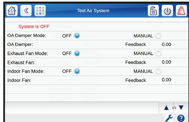
Fig. B — Test DX Circuit and Test Air System Screens (Component Test)
