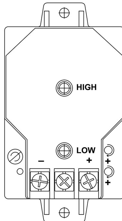
**Fig. 58 – Duct Pressure Transducer**
