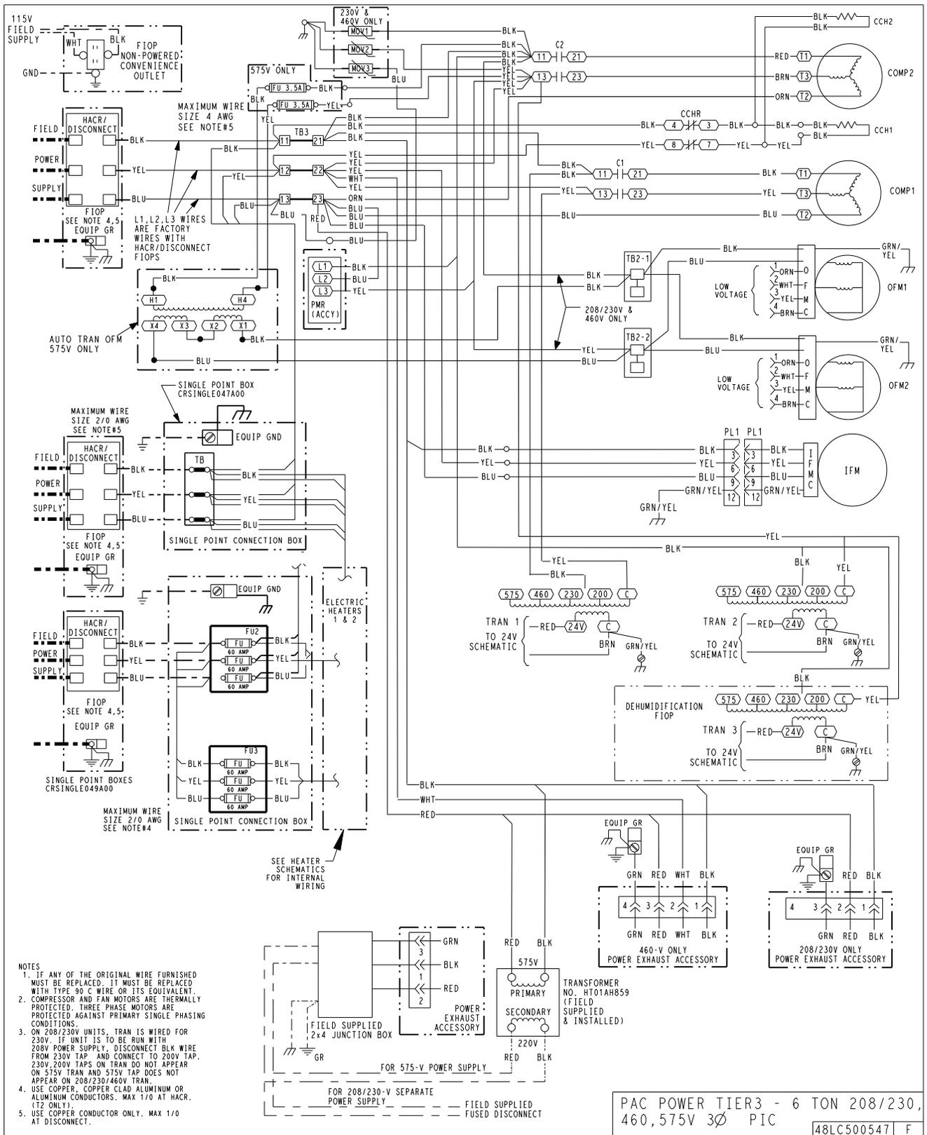
Fig. 38 — 48LC\*H 07 Power Wiring Diagram (208/230-v, 460-v, 575-v Units)
