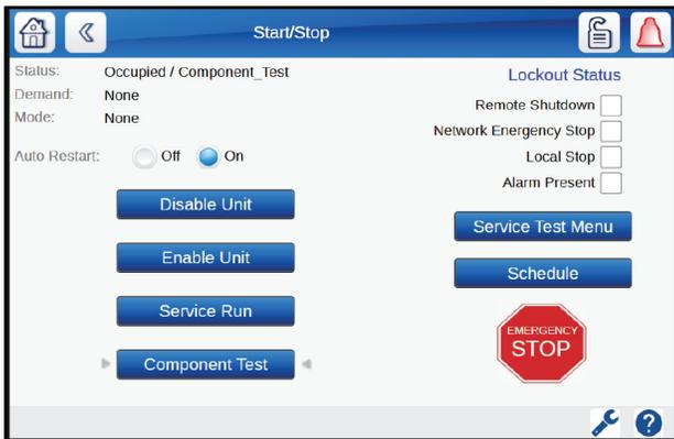
Fig. A — Start/Stop Screen in Test Mode
