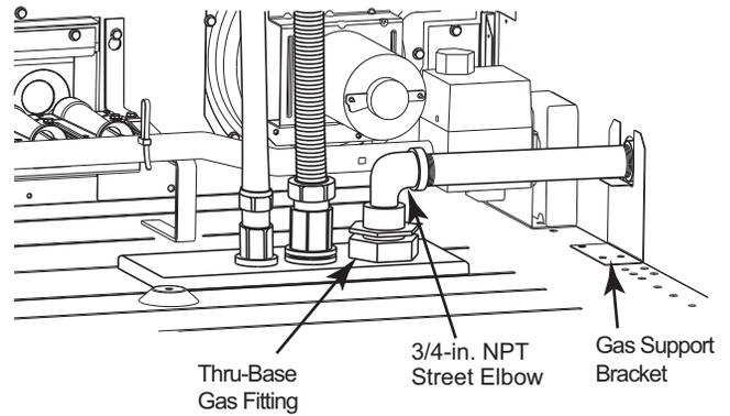
**Fig. 26 — Gas Line Piping**
