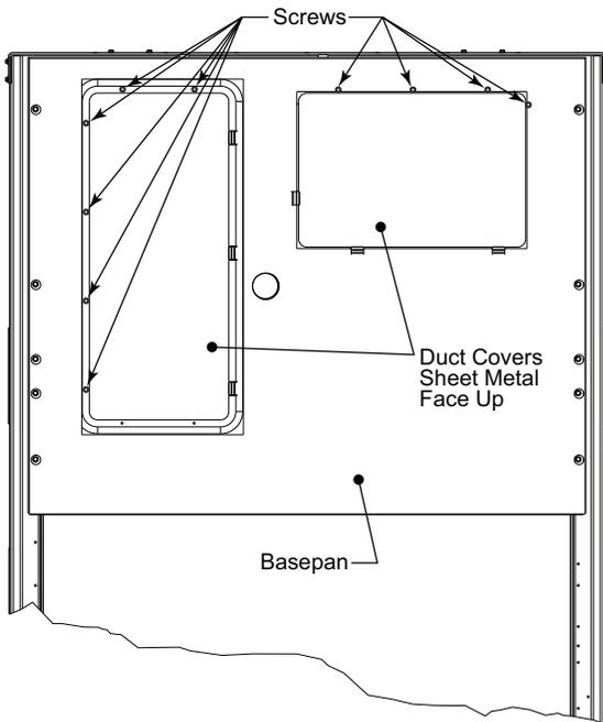
Fig. 13 — Horizontal Duct Panels In Place
