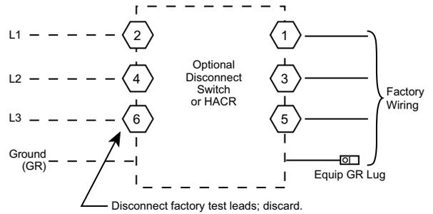
**Units With Electric Heat Option with Single Point Box and Without Disconnect or HACR Option**
