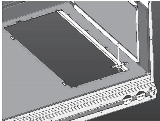
Fig. 14 — SAT Sensor Install Locations
