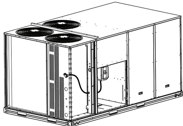
**Fig. 33 — Conduit into Factory Option Non-Fused Disconnect (NFD) or HACR**
