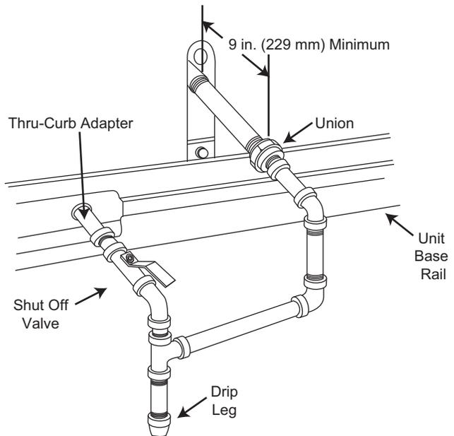
**Fig. 27 — Gas Piping with Direct Drip Leg**
