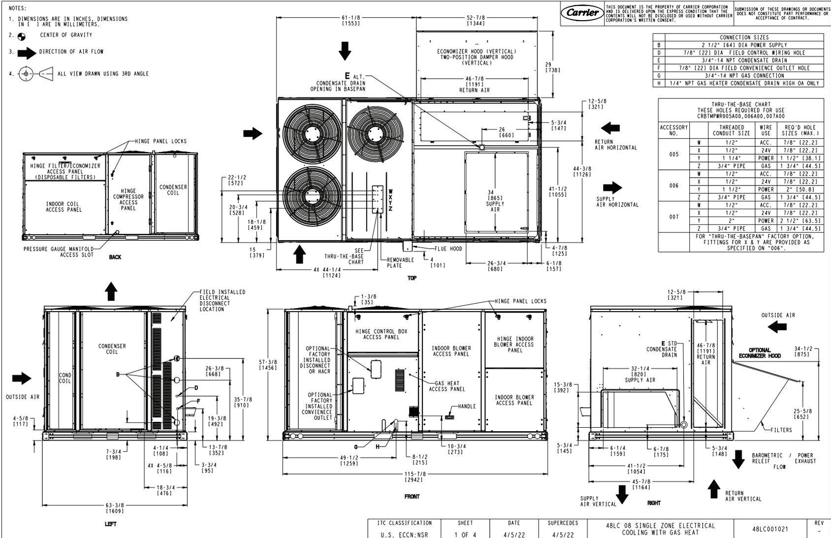
Fig. 3 – Unit Dimensional Drawing, Size 08, Single-Zone Electric Cooling with Gas Heat
