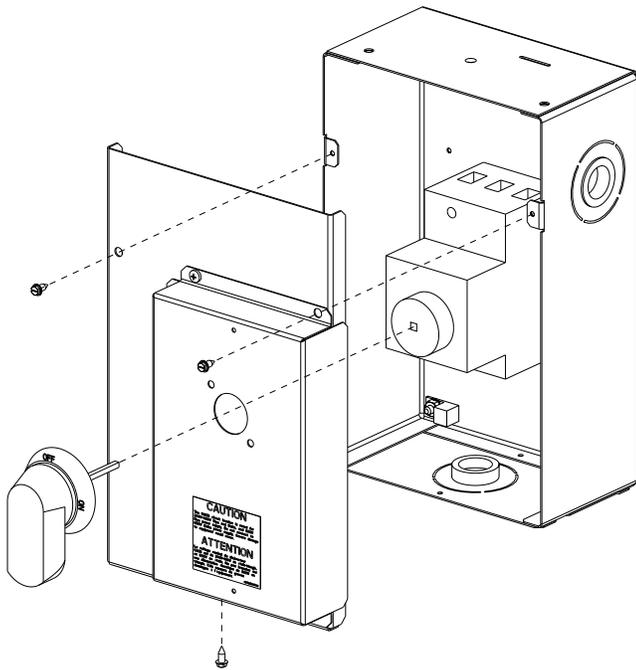
**Fig. 46 — Handle and Shaft Assembly for HACR**
