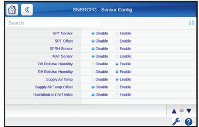
**Fig. 87 — Sensor Configuration Screen Layout**
