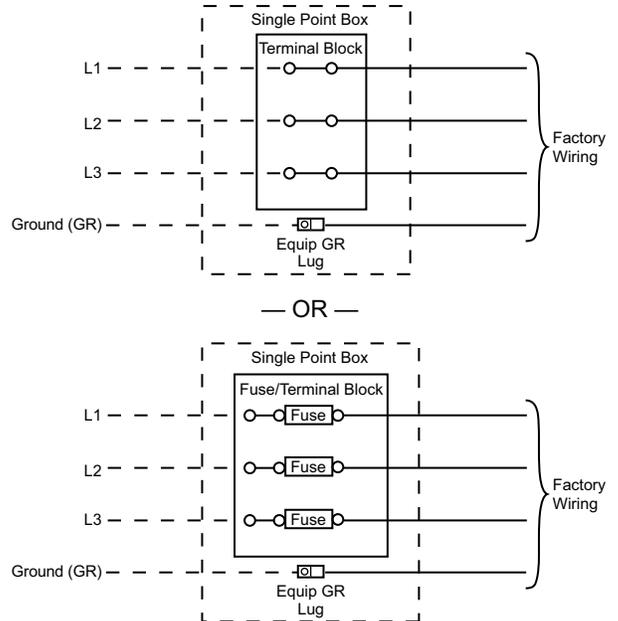
**Fig. 41 — Power Wiring Connections**
