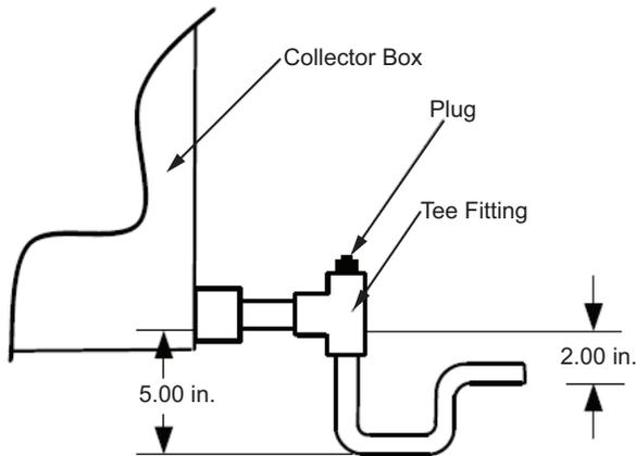
**Fig. 32 — Gas Heater Condensate Drain Example**
