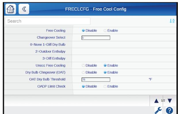
**Fig. 94 — Free Cooling Configuration Screen**
