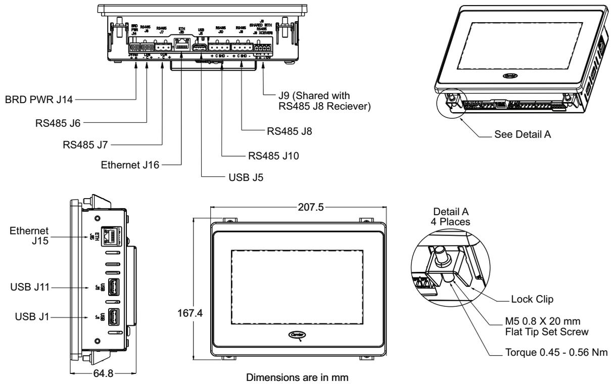
**Fig. 65 – Carrier SmartVu™ Touchscreen Display Interface and Connections**
