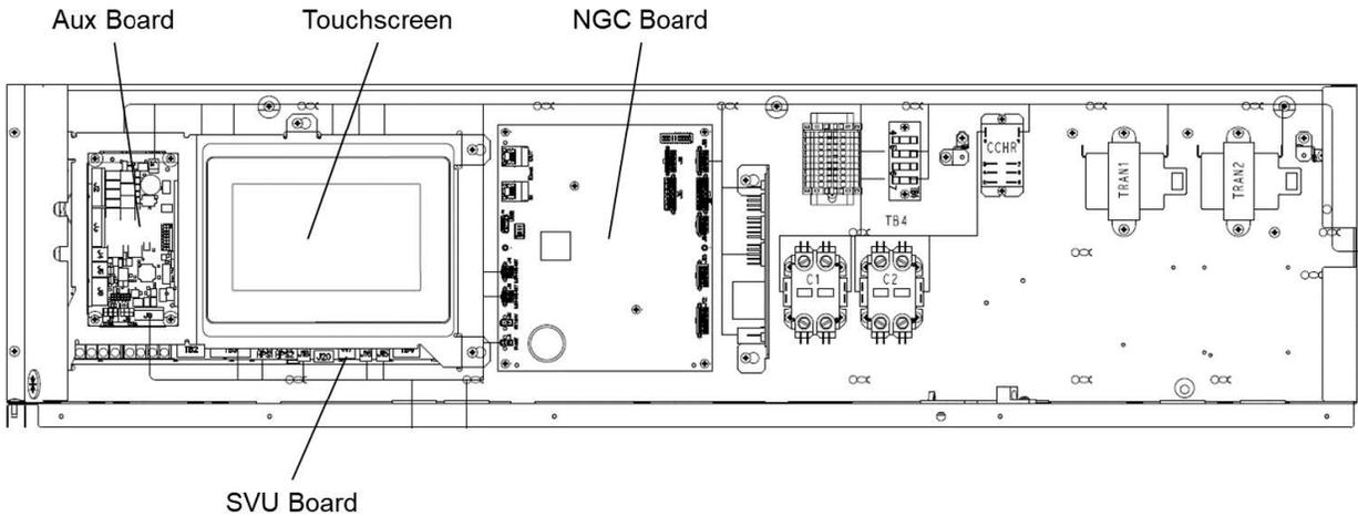
**Fig. 64 — Typical Control Box Layout**
