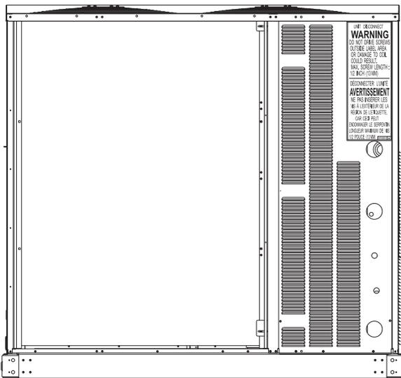
**Fig. 40 — Mounting Position for Field Disconnects (up to 100A)**
