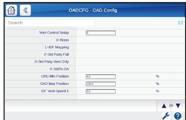
**Fig. 89 – Outdoor Air Damper Configuration Screen**
