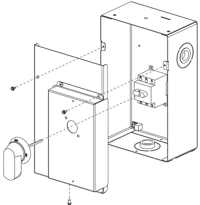
**Fig. 45 — Handle and Shaft Assembly for NFD**
