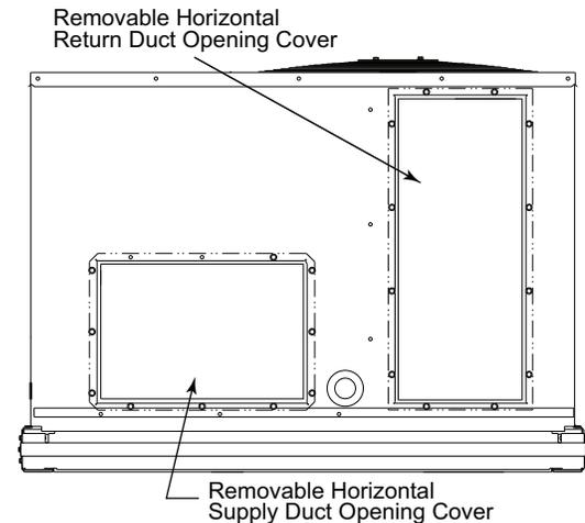
**Fig. 10 — Horizontal Conversion Panels**
