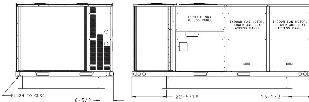
**Fig. 11 — Retrofit Installation Dimensions**
