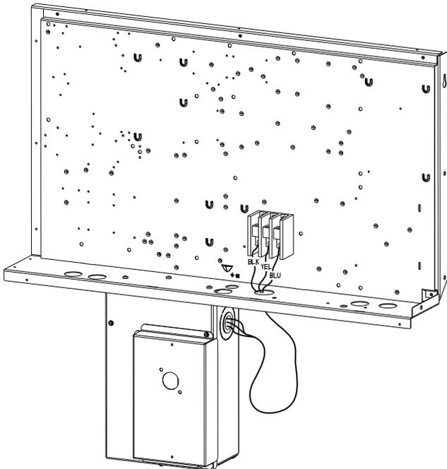
**Fig. 43 — Location of Non-Fused Disconnect (NFD) Enclosure**
