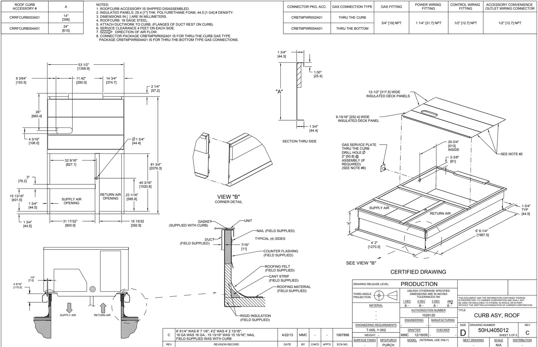
Fig. 6 – Roof Curb Details, Size 07 Units
