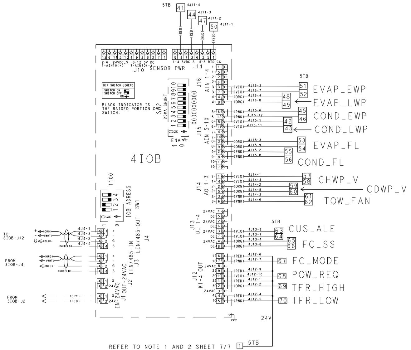
THIS TYPICAL DRAWING SHOWS THE CARRIER STANDARD PRESSURE TRANSDUCER WHICH IS 5VDC POWER SUPPLY.
