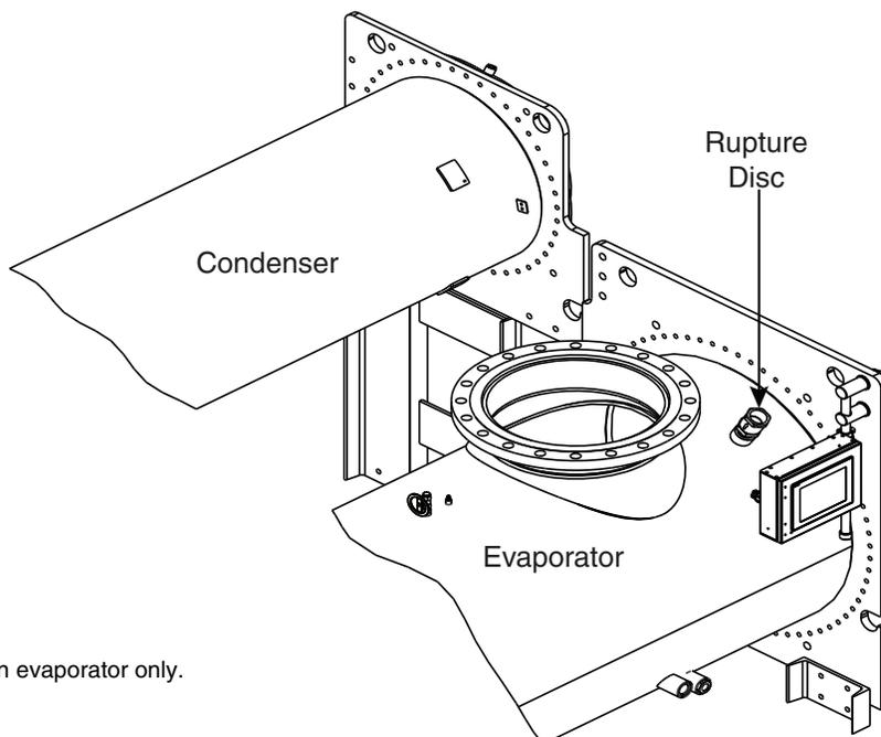
NOTE: Relief valve device on evaporator only.
