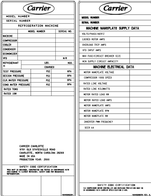
Fig. 1 — 19DV Refrigeration Machine Nameplate
