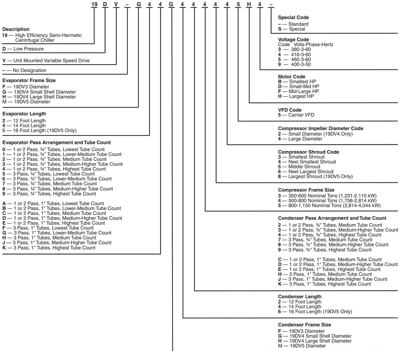
**Fig. 2 — 19DV Chiller Model Number Identification**
