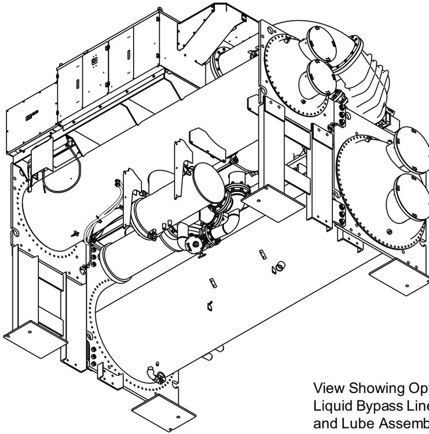
View Showing Optional Economizer Liquid Bypass Line (Control Panel, Purge, and Lube Assembly Removed)
