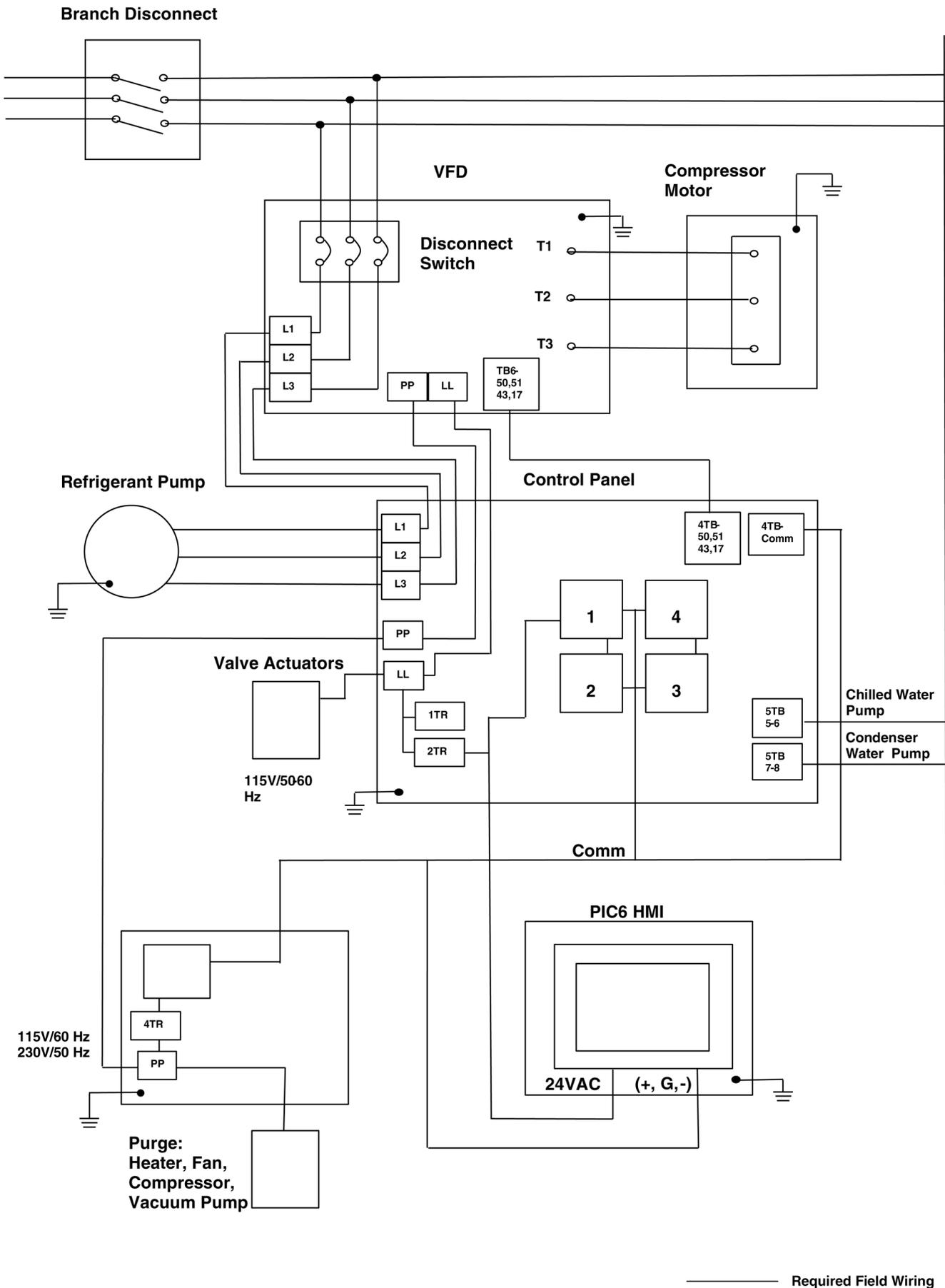
Fig. 27 — Typical 19DV VFD — Factory Unit Mounted
