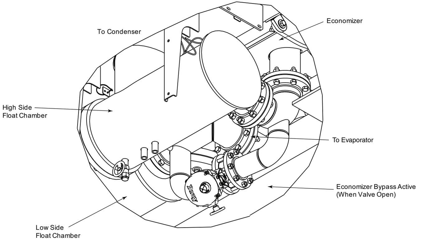
Fig. 4 — Typical 19DV Compressor Chiller Liquid Bypass
