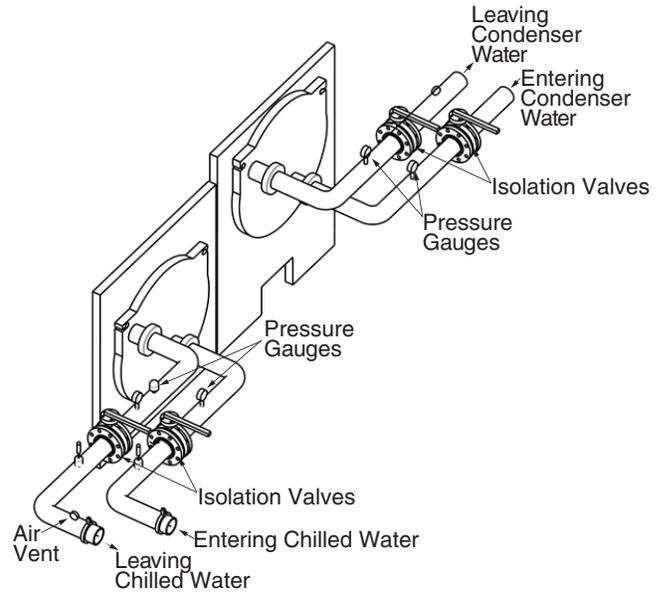
Fig. 14 — Typical Nozzle Piping
