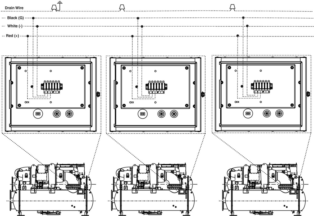
NOTE : Field-supplied terminal strip must be located in control panel.
