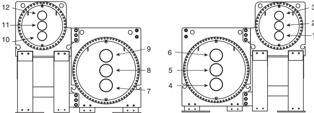
NOZZLE ARRANGEMENT CODES FOR 19DV NOZZLE-IN-HEAD WATERBOXES
