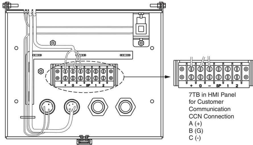
**Fig. 20 — HMI Panel**
