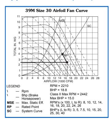
Airflow with a clean filter will be 16,700 cfm. Since airfoil fans are non-overloading (bhp lines run parallel with rpm lines) the bhp does not change (actually, bhp decreases).
