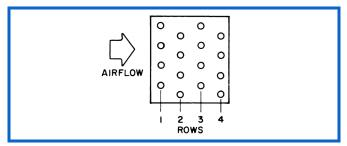
Cooling coils are typically available in 4, 6, 8, and 10-row configurations. Tubes should have an outside diameter (OD) of 1/2 in. to maximize heat transfer at minimum water flows. Coils should be sized for the most efficient use of water. Water temperature differences of 12 to  $16^{\circ}F$  are typical and represent optimum selection points.
