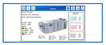
Single-zone cooling and heating demands can be established based on an accessory space temperature (SPT) sensor or 2-stage heat/cool thermostat inputs.
