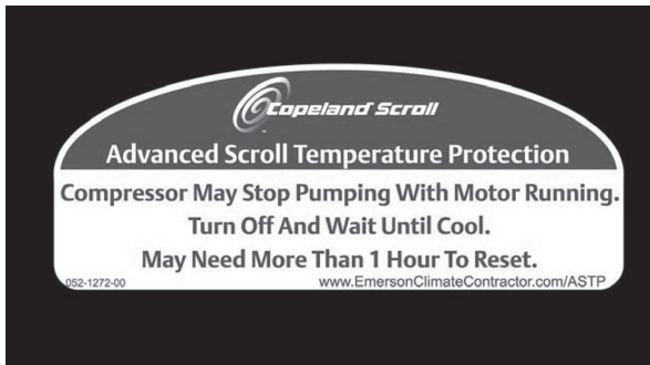
Fig. 18 — Advanced Scroll Temperature Protection Label
