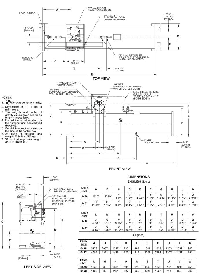
Fig. 27 — Optional Pumpout Unit and Storage Tank
