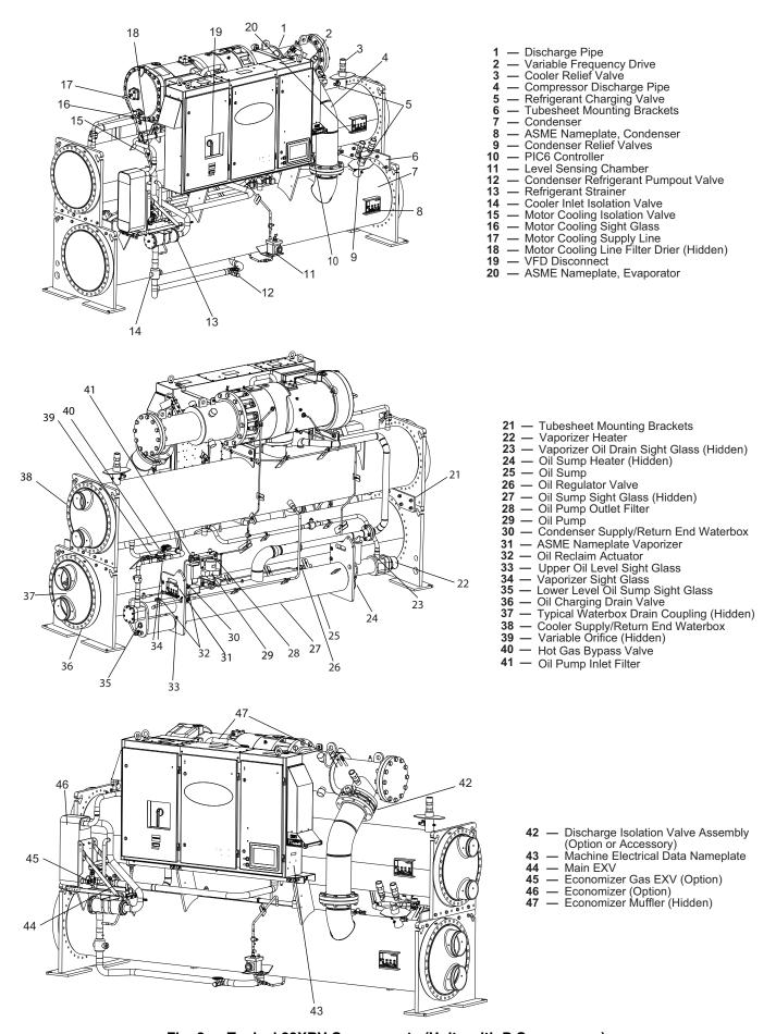
Fig. 2 — Typical 23XRV Components (Units with P Compressor)
