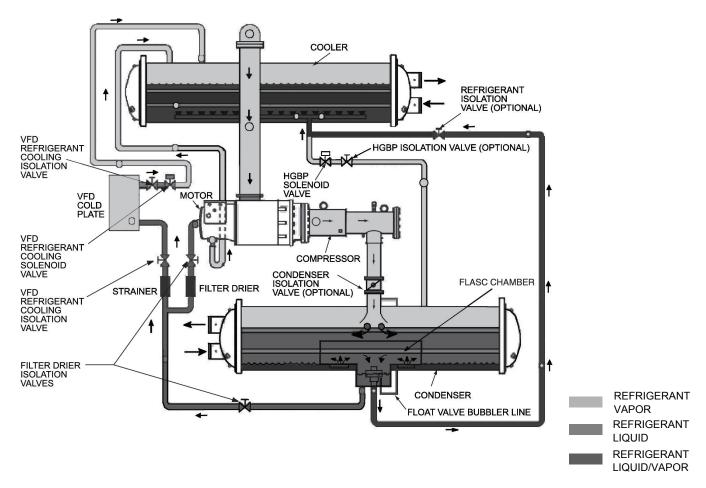
Fig. 9 — Refrigerant Flow Schematic, Q and R Compressors (Without Optional Flash Economizer)
