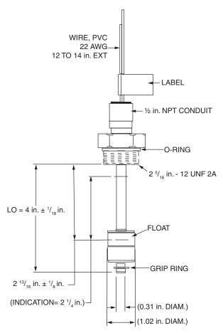
Fig. 61 — Condenser Liquid Level Sensor
