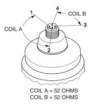
Fig. 60 — EXV Motor Windings Resistance
