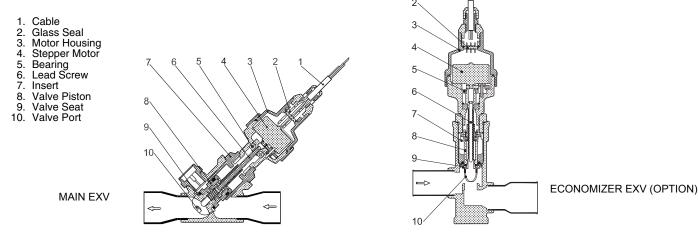
Fig. 21 — Cutaway Views of Electronic Expansion Valves (EXV) (P Compressor Only)
