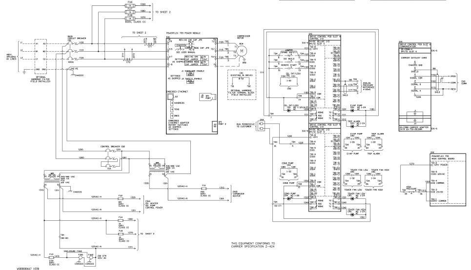
Fig. 64 — 23XRV VFD Schematic (Rockwell Standard Tier VFD)
