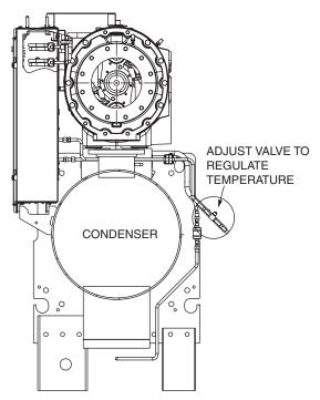
Fig. 31 — Isolation Valve, Leaving Refrigerant Cooling Line
