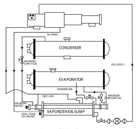
Fig. 13 — Oil Flow Schematic
