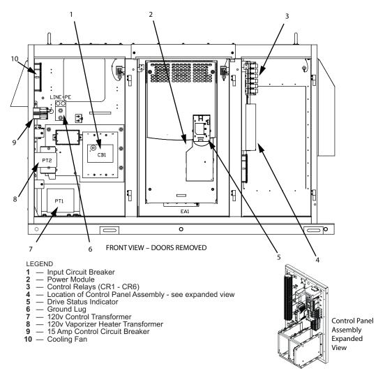
Fig. 18 — Control Center VFD Input Components (Std Tier VFD)
