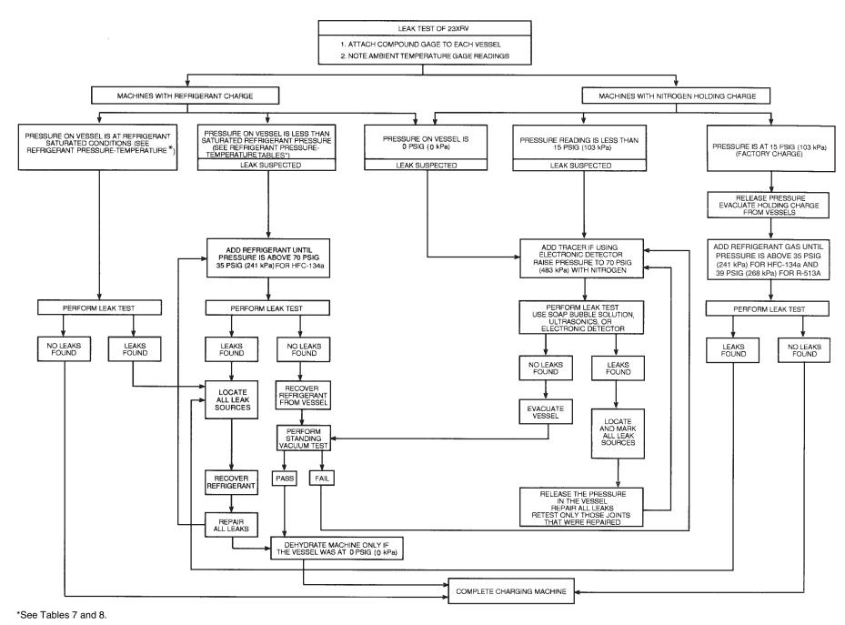
Fig. 26 — 23XRV Leak Test Procedure
