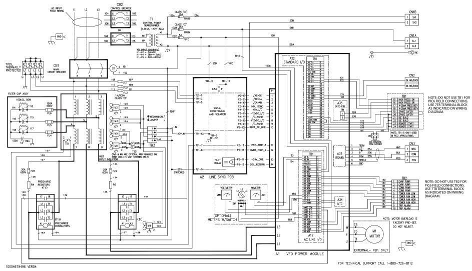
Fig. 63 — 23XRV VFD Schematic (LF-2)
