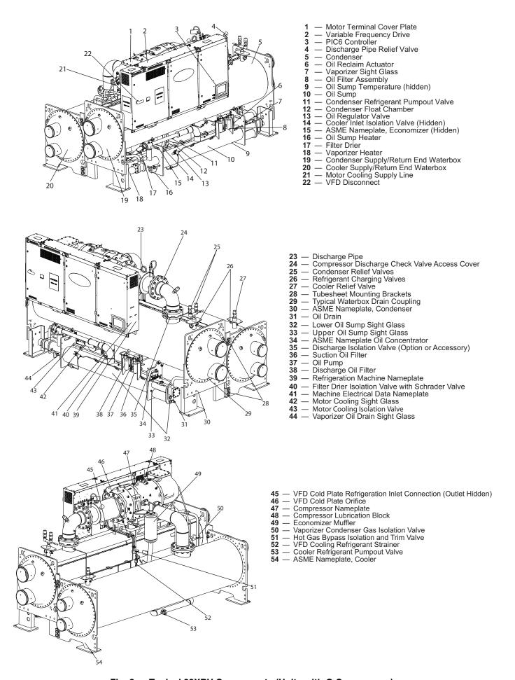
Fig. 3 — Typical 23XRV Components (Units with Q Compressor)
