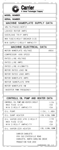
Fig. 32 — Machine Electrical Data Nameplate
