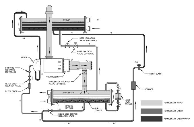
Fig. 10 — Refrigerant Flow Schematic, P Compressor (Without Optional Economizer)
