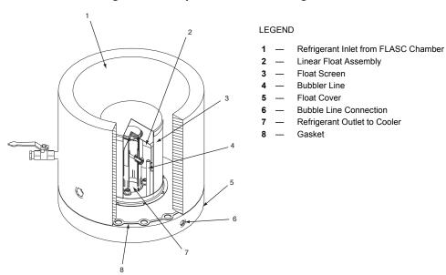
Fig. 56 — 23XRV Float Valve Design (Frame 3-5 Heat Exchangers Only)
