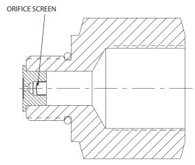
Fig. 55 — Compressor Inlet Bearing Oil Orifice
