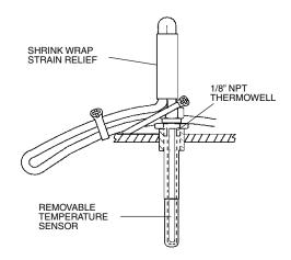
Fig. 14 — Control Sensors (Temperature)
