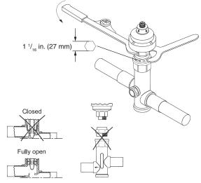
Fig. 58 — EXV Disassembly
