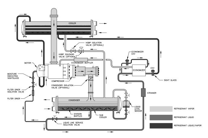
Fig. 12 — Refrigerant Flow Schematic, P Compressor (With Optional Economizer)
