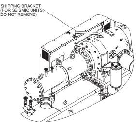
Fig. 45 — Control Center Shipping Bracket (Unit with R Compressor Shown)
