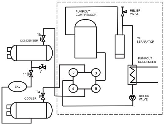
Fig. 51 — Pumpout System Piping Schematic without Storage Tank for 23XRV Units with P Compressor
