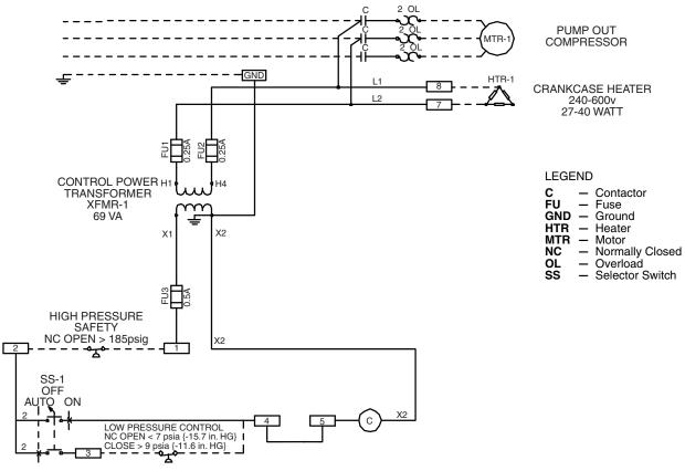
Fig. 48 — 23XRV Pumpout Unit Wiring Schematic
