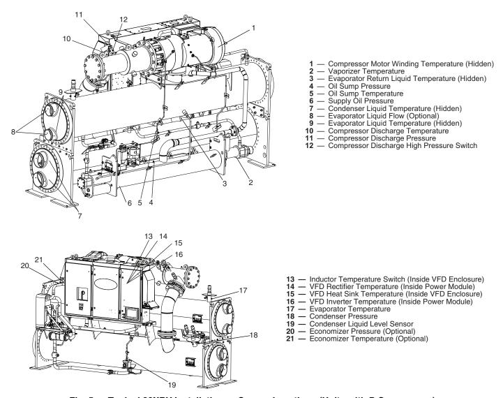
Fig. 5 — Typical 23XRV Installation — Sensor Locations (Units with P Compressor)
