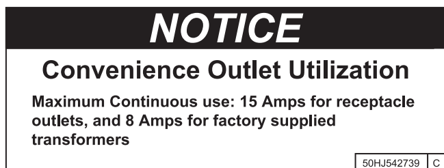
Fig. 30 — Convenience Outlet Utilization Notice Label
