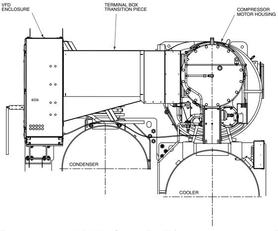
Fig. 23 — 900A or 1200A LF2 VFD or Standard Tier VFD (765, 855, 960, 1070, 1275, 1530A)
