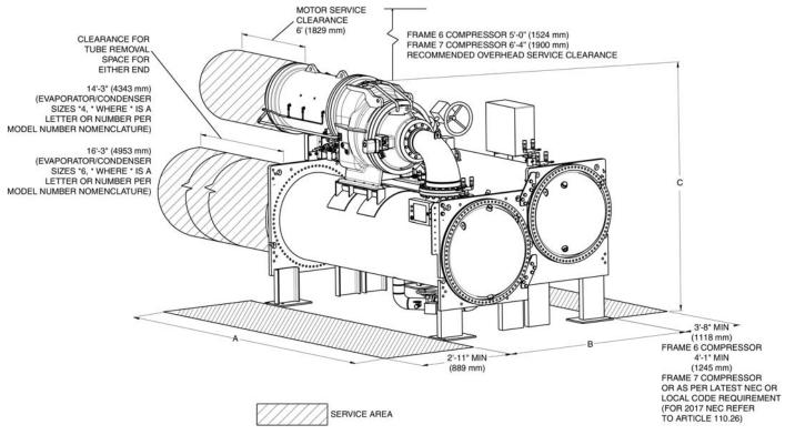
NOTE: Compressor Frame Size 6, dished head waterbox shown.
