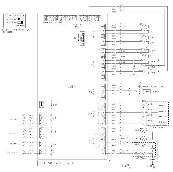
Fig. 67 — 19XR6-7 Chiller Control Schematic
