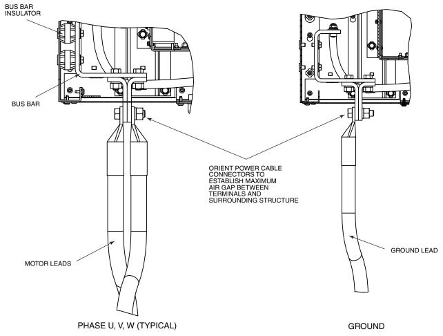
Fig. 25 — Motor Lead Installation (View Looking Down)
