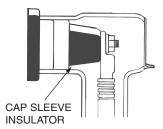
Fig. 69 — Cap Sleeve Insulation to Prevent Arcing
