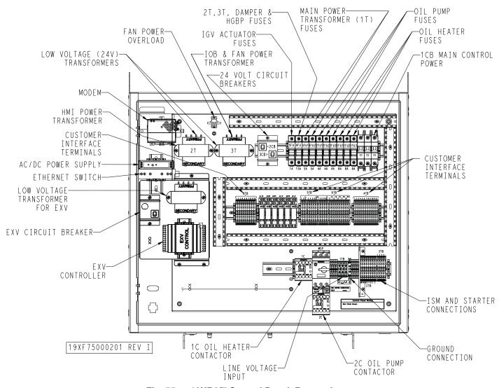
Fig. 55 — 19XR6/7 Control Panel, Bottom Layer
