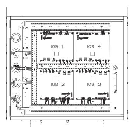
Fig. 54 — 19XR6/7 Control Panel, IOB Layer
