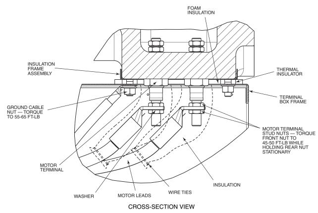
Fig. 24 — Compressor Motor Terminals (Typical)
