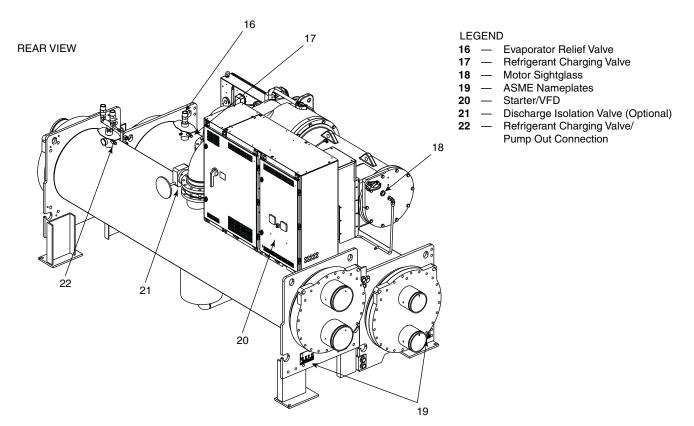
Fig. 4 — 19XR,XRV Single-Stage Compressor, Frame Size 2, 3, 4, 5
