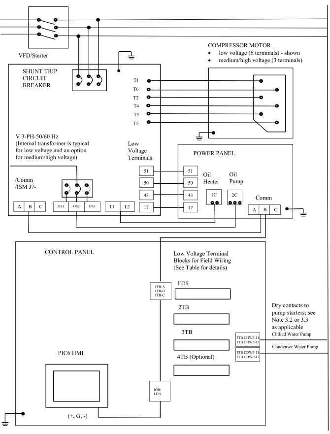
Fig. 59 — 19XR2-E with Benshaw Free-Standing Starter with MX3 Modbus Communication
