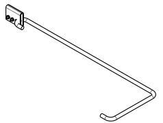
Fig. 47 — Circuit Breaker Handle Extension
