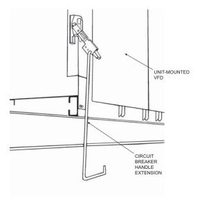
Fig. 48 — Circuit Breaker Handle Extension Installed
