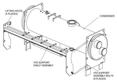
Fig. 28 — 900A or 1200A VFD Support Assembly Installation
