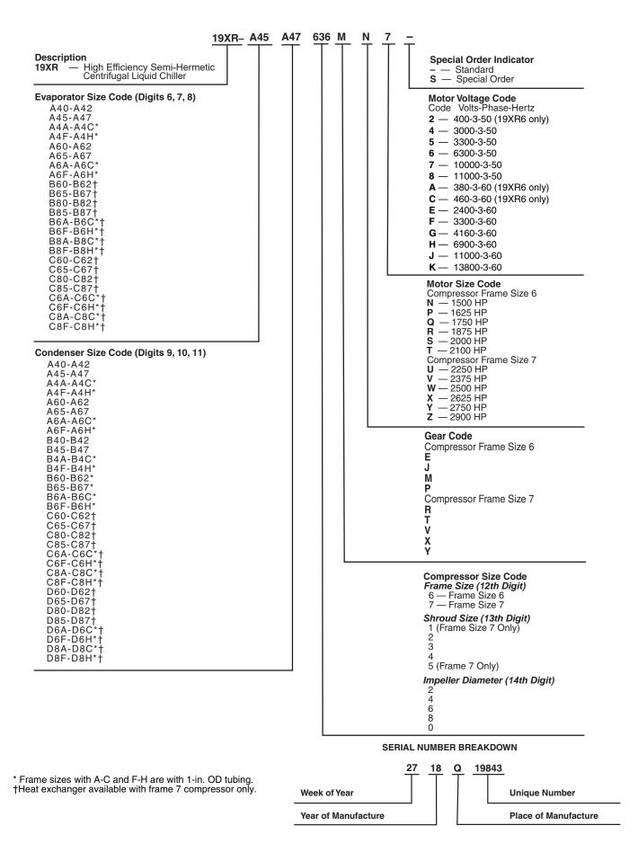
Fig. 3 — 19XR Two-Stage Compressor Frame Size 6 and 7
