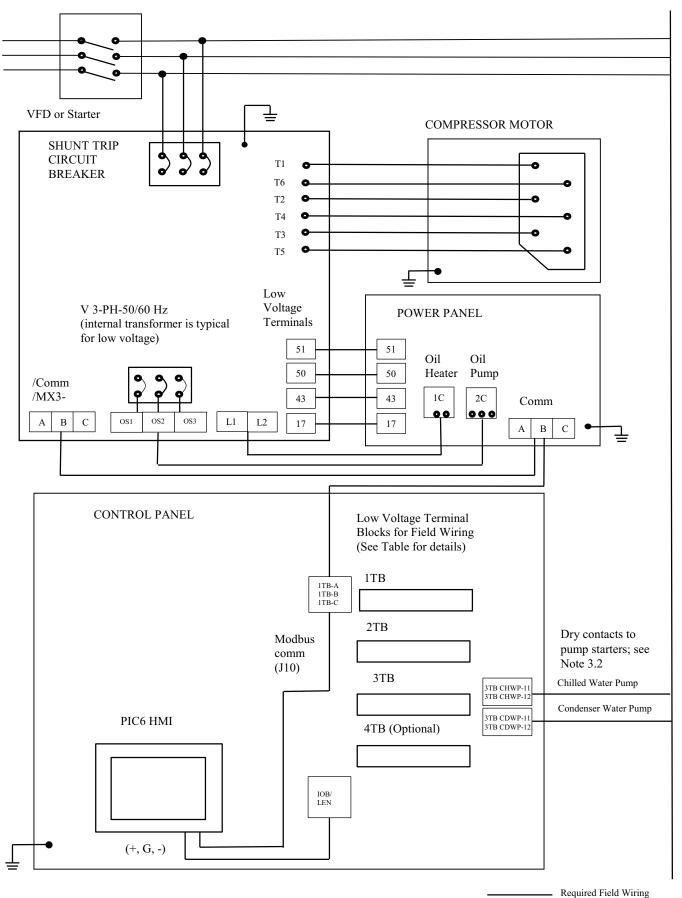
Fig. 58 — Typical 19XR2-E Fixed Speed or VFD — Factory Unit Mounted (Low Voltage)
