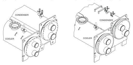
Fig. 44 — 19XR Relief Valve Arrangements
