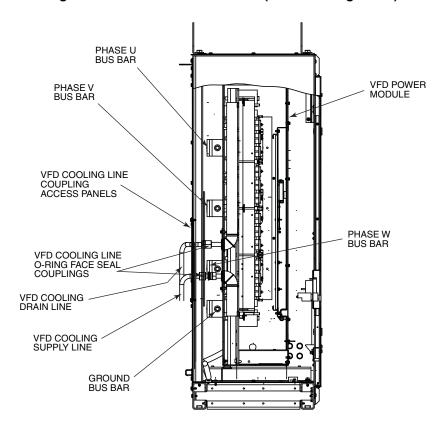
Fig. 26 — 900A or 1200A VFD Refrigerant Cooling Lines
