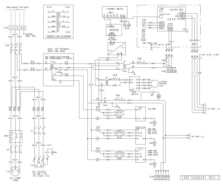
Fig. 66 — 19XR6-7 Controls Diagram
