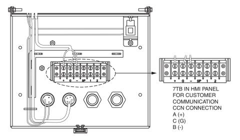
Fig. 53 — 19XR6/7 HMI Panel
