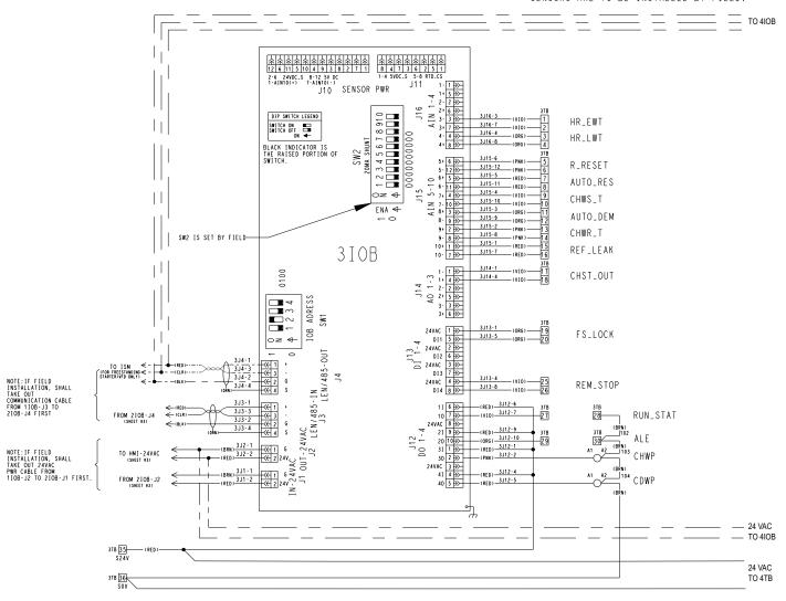
Fig. 61 — 19XR2-E Chiller Control Schematic (cont) FIELD TERMINALS for 3TB, Fig. 61
