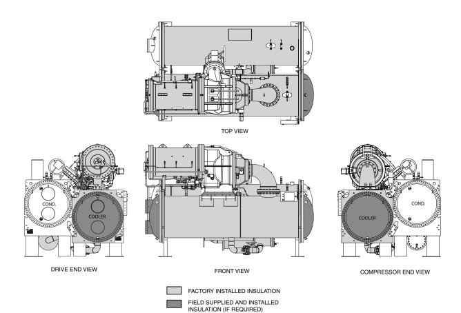
Fig. 70 — 19XR Insulation Area (Typical Unit with Economizer)
