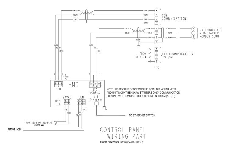
Fig. 61 — 19XR2-E Chiller Control Schematic (cont)
