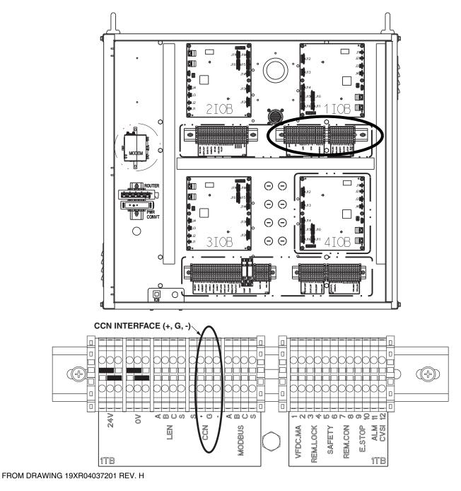
Fig. 50 — 19XR2-E Control Panel — CCN Communication Wiring for Multiple Chillers
