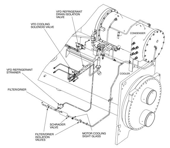
Fig. 21 — 900A or 1200A LF2 VFD or Standard Tier VFD (765, 855, 960, 1070, 1275, 1530A) Isolation Valves — Typical
