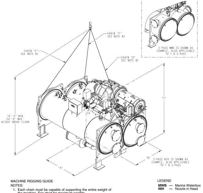
Each chain must be capable of supporting the entire weight of the machine. See chart for maximum weights.
