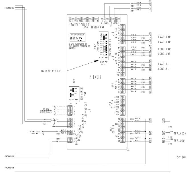
Fig. 61 — 19XR2-E Chiller Control Schematic (cont) FIELD TERMINALS for 4TB, Fig. 61
