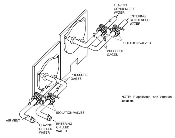
Fig. 38 — Typical Nozzle Piping
