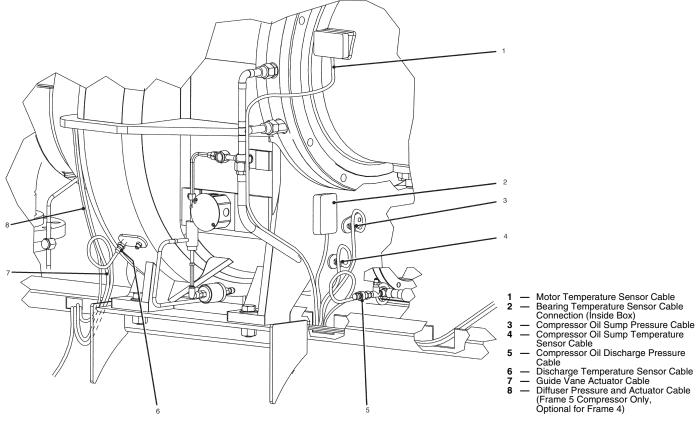
Fig. 19 — Compressor Detail
