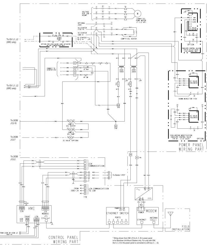
Fig. 62 — 19XR2-E Chiller Control Schematic for Non-Unit Mount VFD Chiller (Fixed Speed Chiller and free-standing VFD)
