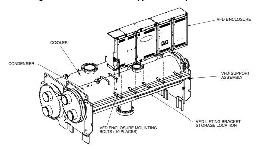
Fig. 29 — 900A or 1200A VFD Enclosure Installation
