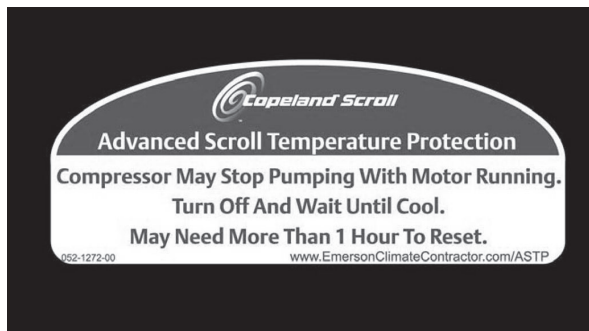
Fig. 14 — Advanced Scroll Temperature Protection Label
