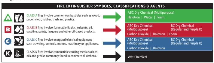
**NOTE:** Although ABC and BC Dry Chemical extinguishers can control fires involving electronic equipment, the National Fire Protection Association Standard for portable extinguishers (NFPA-10) advises against dry chemical extinguishers for fires involving delicate electronic equipment due to potential damage and clean up issues presented with agent residues.
