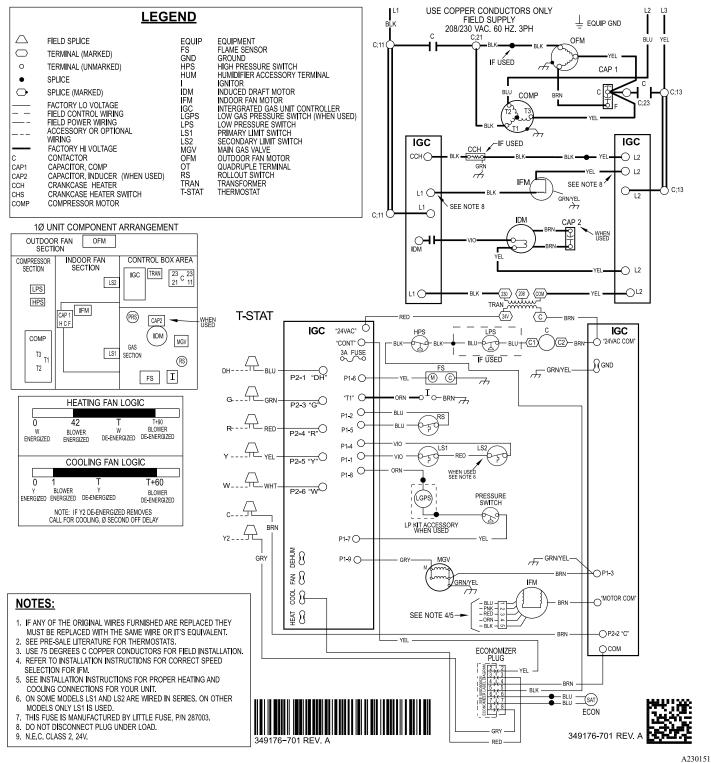
Fig. 17 – 208/230-3-60 Ladder Wiring Diagram
