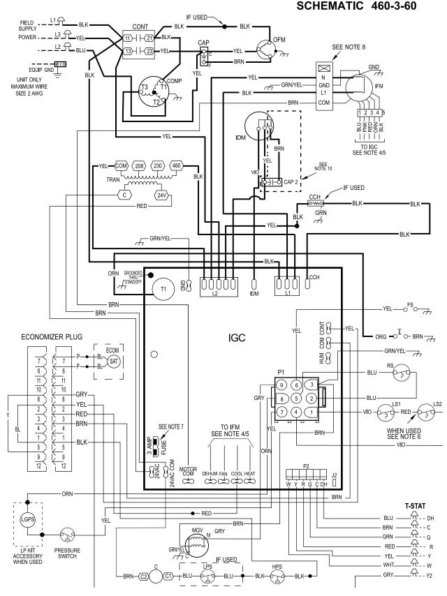
Fig. 18 – 460-3-60 Connection Wiring Diagram
