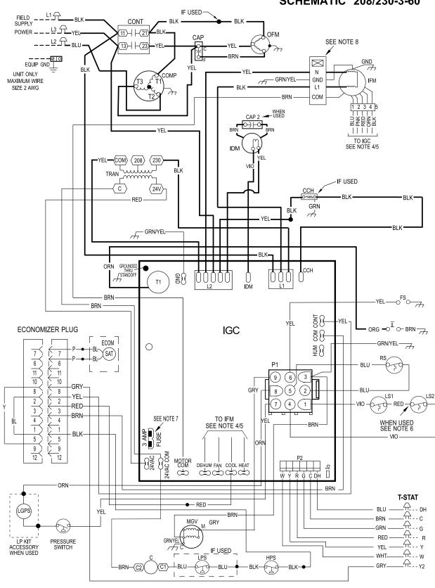
Fig. 16 – 208/230-3-60 Connection Wiring Diagram
