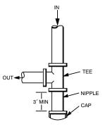
Fig. 8 – Sediment Trap
