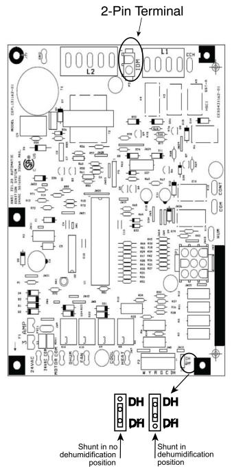
Fig. 19 - Ultra Low NOx Single Phase IGC Board
