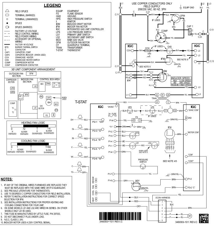
Fig. 18 – 208/230-3-60 Ultra Low NOx Ladder Wiring Diagram
