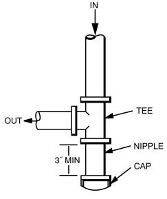
Fig. 8 – Sediment Trap
