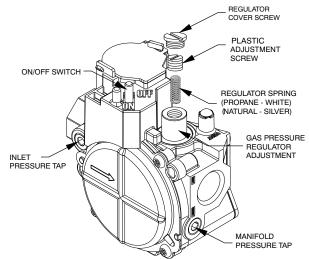
Fig. 13 – Standard Single-Stage Gas Valve
