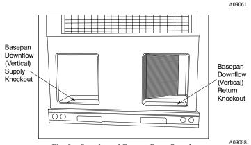
Fig. 9 – Supply and Return Duct Opening
