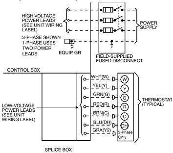
Fig. 10 - High- and Control-Voltage Connections
