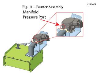
Fig. 12 – BurnerBox/Gas Manifold Assembly
