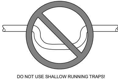
Fig. 19 – Insufficient Condensate Trap
