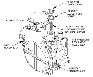
Fig. 13 - Standard Single-Stage Gas Valve
