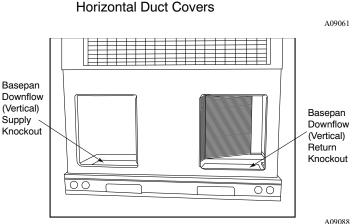
Fig. 9 - Supply and Return Duct Opening
