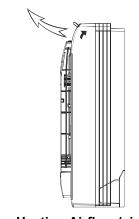
Fig. 16 — Heating Airflow (sizes 09-12)
