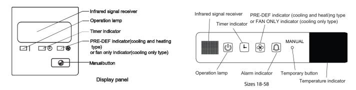
Fig. 2 — IR (Infrared) Receiver Display Panel
