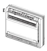
Fig. 18 — Louver Up-Down Swing (Sizes 09-12)
