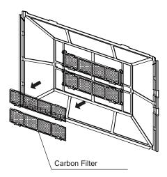
Fig. 30 — Carbon Filter
