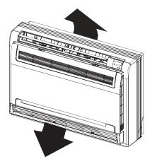
Fig. 23 — Air Blows from Upper and Lower Outlets
