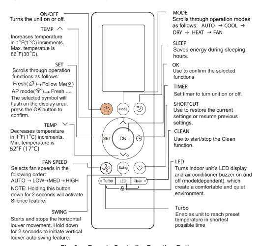
Fig. 3 — Remote Controller Function Buttons
