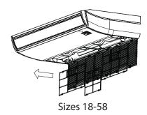
Fig. 29 — Remove the air filter
