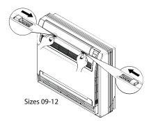
Fig. 25 — Open the front panel
