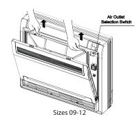
Fig. 27 — Remove the air filter
