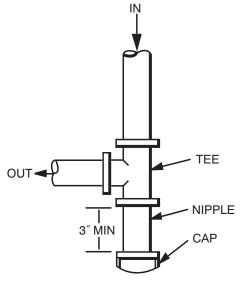
Fig. 8 - Sediment Trap
