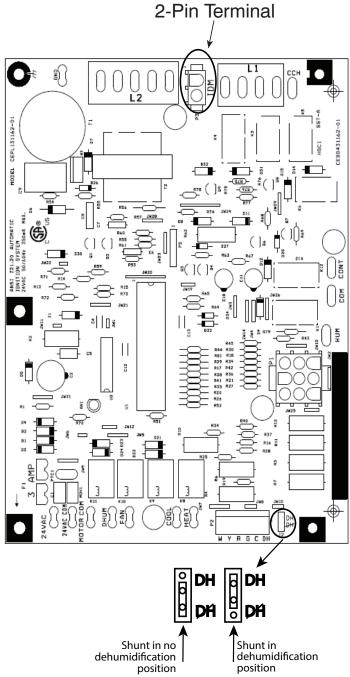
Fig. 19 - Ultra Low NOx Single Phase IGC Board
