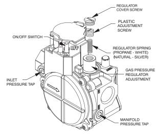
Fig. 13 – Standard Single-Stage Gas Valve
