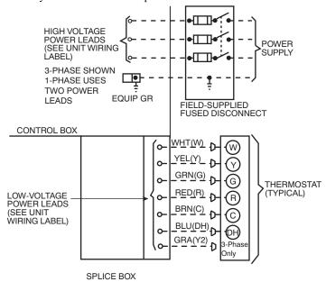
Fig. 10 – High- and Control-Voltage Connections
