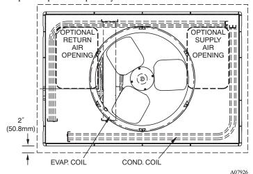
Fig. 2 - Slab Mounting Details
