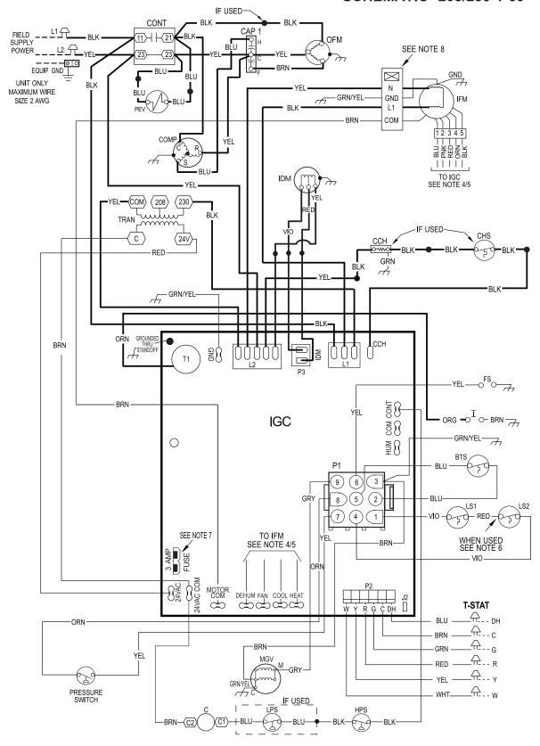
Fig. 15 – 208/230-1-60 Ultra Low NOx Connection Wiring Diagram
