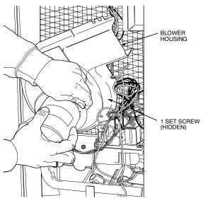
Fig. 23 – Removal of Motor and Blower Wheel
