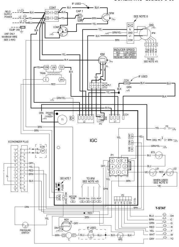
Fig. 17 – 208/230-3-60 Ultra Low NOx Connection Wiring Diagram
