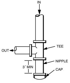
Fig. 8 – Sediment Trap
