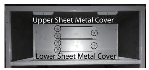
Fig. 4 — Remove Sheet Metal Covers
