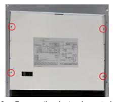
Fig. 8 — Remove the electronic control box
