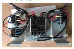
Fig. 12 — Secure the power input wires of each group
