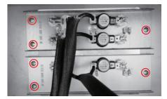
Fig. 6 — Install the Electric Heating Module
