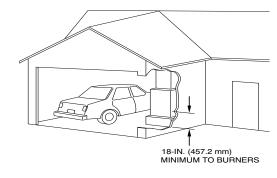
Fig. 5 – Installation in a Garage
