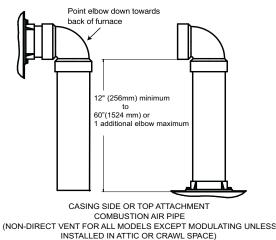
Fig. 47 – Combustion Air Pipe Attachment
