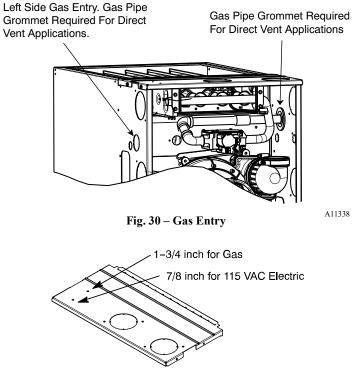
Fig. 31 – Alternate Gas and Electric Entry
