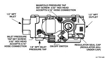
Fig. 64 – Gas Valve with Tower Pressure Ports
