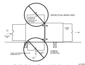
Fig. 23 – Horizontal Return Air Configurations and Restrictions
