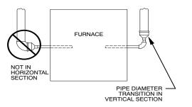
Fig. 50 – Combustion Air and Vent Pipe Diameter Transition<sup>A93034</sup> Location and Elbow Configuration
