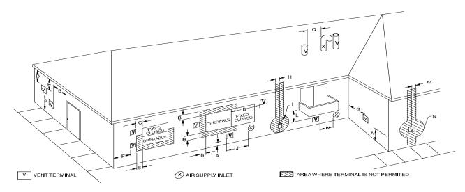
Fig. 43 – Direct Vent Termination Clearance
