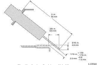
Fig. 69 – Igniter Position - Side View
