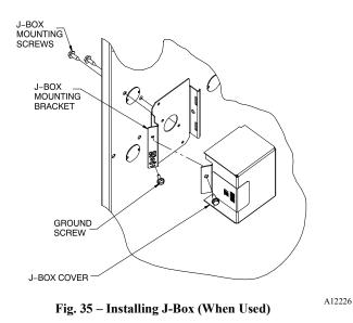
The J-Box cover, mounting bracket and screws are shipped in the loose parts bag included with the furnace. See Fig. 35 for J-Box mounting locations.
