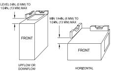
Fig. 19 – Furnace Pitch Requirements
