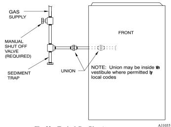
Fig. 32 – Typical Gas Pipe Arrangement
