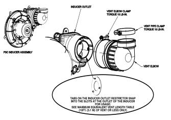
Fig. 53 – Inducer Vent Elbow
