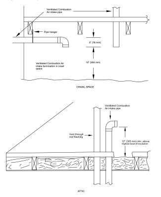
Fig. 48 – Vent Terminations for Ventilated Combustion Air
