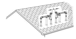
Fig. 46 – Pipe Vent and Combustion Ventilated Combustion Air
