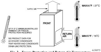
Fig. 3 – Freeze Protection and Return Air Temperature
