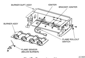
Fig. 67 – Burner Assembly
