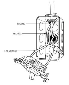
**Fig. 36 – Field-Supplied External Electrical Box on Furnace Casing NOTE:** If electrical entry through the furnace top panel is used, mark the screw hole locations using the mounting holes in the external electrical box as a template.
