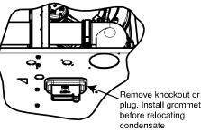
Fig. 18 – Horizontal Drain Trap Grommet
