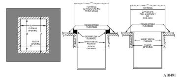
Fig. 25 – Installation on Combustible Flooring
