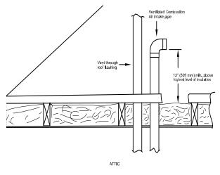
Fig. 48 – Vent Terminations for Ventilated Combustion Air
