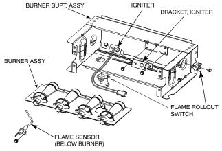
Fig. 67 – Burner Assembly
