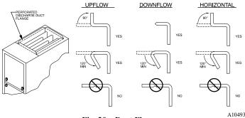
Fig. 20 - Duct Flanges
