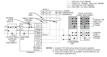
Fig. 33 - Typical Field Wiring Diagram
