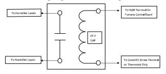
Fig. 37 – Field-supplied Isolation Relay for Humidifiers with
