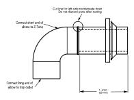
Fig. 17 – Modify Rubber Drain Elbow
