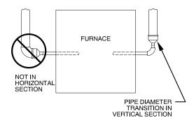
Fig. 50 – Combustion Air and Vent Pipe Diameter Transition
