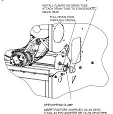
TO 3/4-IN. PVC ADAPTER OR 1/2-IN. CPVC PIPE \*CLAMP MAY BE LOCATED ON OUTSIDE OF DRAIN TUBE
