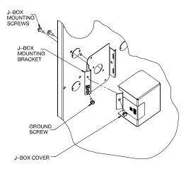
Fig. 35 – Installing J-Box (When Used)
