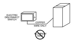
Fig. 34 – Field-Supplied External Electrical Box on Furnace Casing
