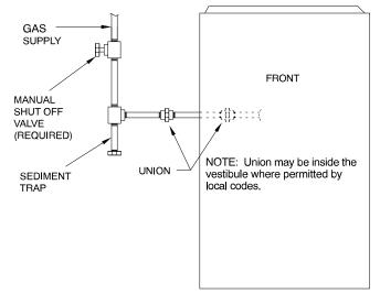
Fig. 32 - Typical Gas Pipe Arrangement
