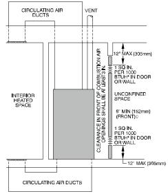
Minimum opening size is 100 sq in. (64516 sq. mm) with minimum dimensions of 3-in. (76mm)
