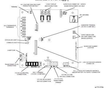
Fig. 38 – Example of Single Stage Furnace Control
