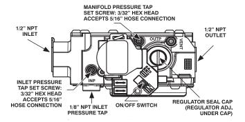
Fig. 64 – Gas Valve with Tower Pressure Ports
