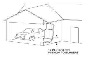
Fig. 5 – Installation in a Garage
