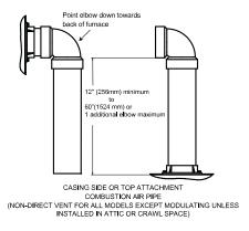
Fig. 47 - Combustion Air Pipe Attachment
