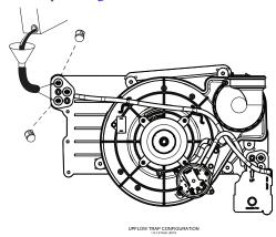
Fig. 62 – Priming Condensate Trap
