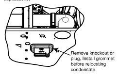
Fig. 18 - Horizontal Drain Trap Grommet
