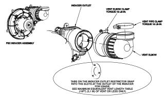
Fig. 53 – Inducer Vent Elbow
