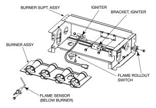
Fig. 68 – Burner Assembly
