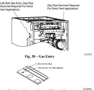
Fig. 31 – Alternate Gas and Electric Entry
