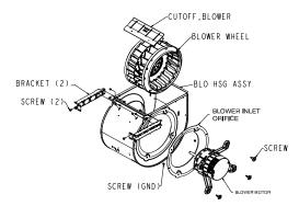
Fig. 66 – Blower Assembly on 040M14--10 and 060M14-- $\overset{\mathrm{Al}90094B}{12}$
