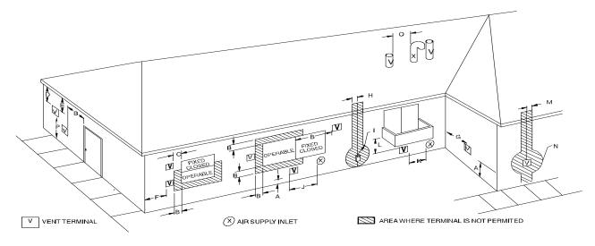
Fig. 43 – Direct Vent Termination Clearance
