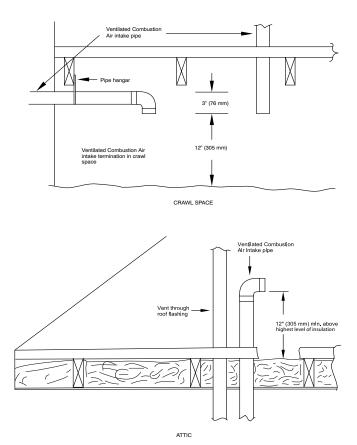
Fig. 47 – Vent Terminations for Ventilated Combustion Air  $^{\rm A10497}$
