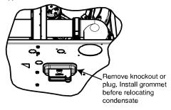
Fig. 18 – Horizontal Drain Trap Grommet
