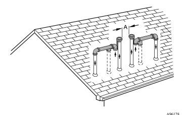
Fig. 48 – Pipe Vent and Combustion
