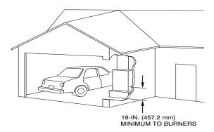
Fig. 5 – Installation in a Garage
