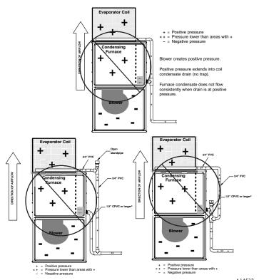
$\textbf{Fig. 13-Example} \ \ \textbf{of Field Drain Attachment (Not Allowed)}^{A14532}$
