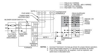
Fig. 33 - Typical Field Wiring Diagram
