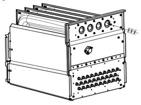
Fig. 71 – Cleaning Heat Exchanger Cell
