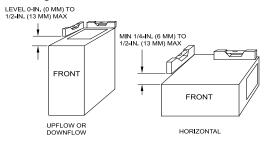
Fig. 19 - Furnace Pitch Requirements
