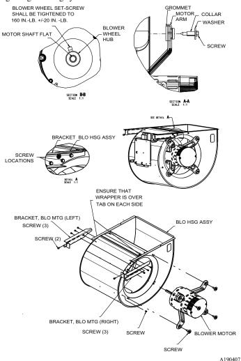
Fig. 67 – Blower Assembly on 100M21--22
