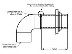
Fig. 17 – Modify Rubber Drain Elbow
