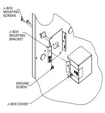
Fig. 35 – Installing J-Box (When Used)
