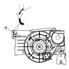
Fig. 62 – Priming Condensate Trap
