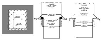
Fig. 25 - Installation on Combustible Flooring
