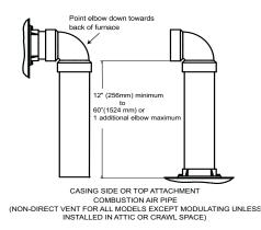
Fig. 46 – Combustion Air Pipe Attachment
