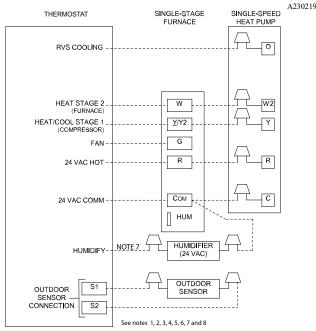
Single-Stage Furnace with Single-Speed Heat Pump
