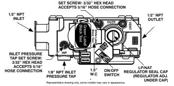
26,000 BTUh Low Capacity Gas Valve with Tower Pressure Ports
