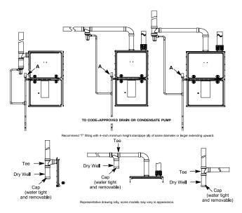
Fig. 51 – Recommended Combustion Air Inlet Moisture Trap
