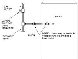
Fig. 32 – Typical Gas Pipe Arrangement
