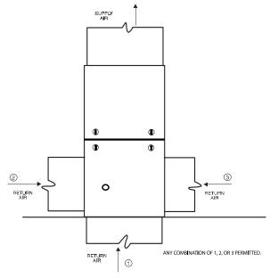
Fig. 21 – Upflow Return Air Configurations and Restrictions  $^{\rm A11036}$
