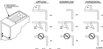
Fig. 20 – Duct Flanges
