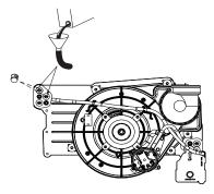
Fig. 62 - Priming Condensate Trap
