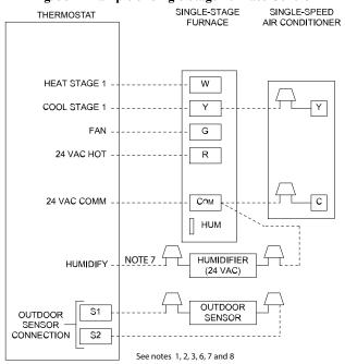
Single-Stage Furnace with Single-Speed Air Conditioner
