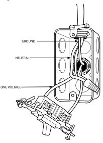
Fig. 36 – Field-Supplied External Electrical Box on Furnace Casing
