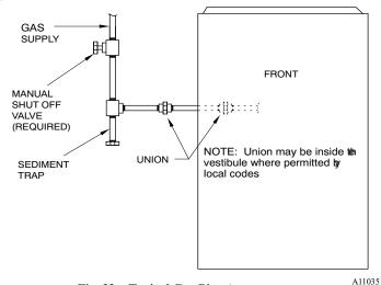
Fig. 32 – Typical Gas Pipe Arrangement
