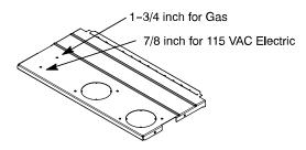
Fig. 31 – Alternate Gas and Electric Entry
