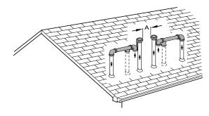
$Fig.\ 46-Pipe\ Vent\ and\ Combustion$
