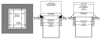
Fig. 25 – Installation on Combustible Flooring
