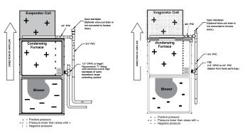
Fig. 12 - Example of Field Drain Attachment
