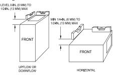
Fig. 19 - Furnace Pitch Requirements
