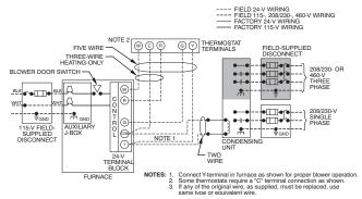
Fig. 33 – Typical Single-Stage Wiring Diagram
