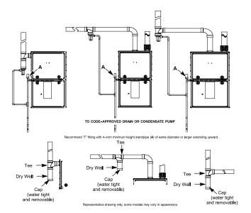
$\textbf{Fig. 51-Recommended Combustion Air Inlet Moisture Trap} \\ \textbf{Air Inlet Moisture Trap} \\ \\ \textbf{Air Inlet Moisture Trap} \\ \textbf{Air Inle$
