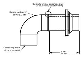
Fig. 17 - Modify Rubber Drain Elbow
