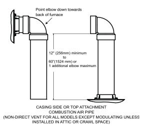
Fig. 47 – Combustion Air Pipe Attachment
