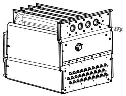
Fig. 70 - Cleaning Heat Exchanger Cell
