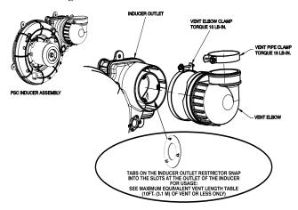
Fig. 53 – Inducer Vent Elbow
