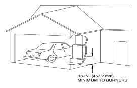
Fig. 5 – Installation in a Garage
