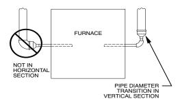
Fig. 50 – Combustion Air and Vent Pipe Diameter Transition A93034 Location and Elbow Configuration
