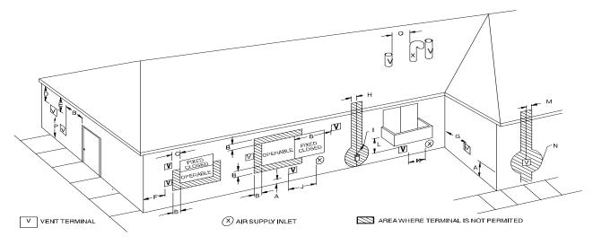
**Fig. 43 – Direct Vent Termination Clearance**
