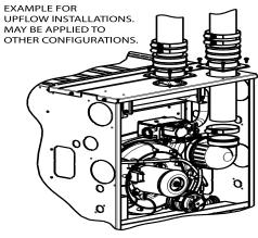
Fig. 45 – Sample Inlet Air Pipe Connection for Polypropylene A122200 Venting Systems
