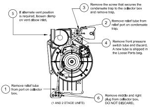
Unconverted Factory Trap Configuration
