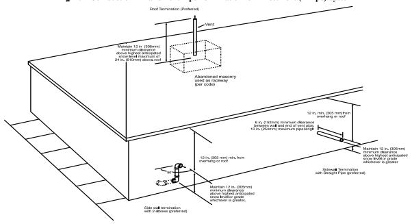
Fig. 41 - Vent Pipe Termination for Non-Direct Vent and Ventilated Combustion Air System
