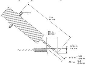
Fig. 69 – Igniter Position - Side View
