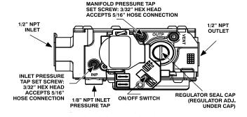
Fig. 64 – Gas Valve with Tower Pressure Ports
