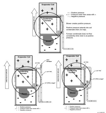
$\textbf{Fig. 13-Example of Field Drain Attachment (Not Allowed)}^{\text{A14532}}$
