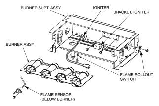
Fig. 67 – Burner Assembly
