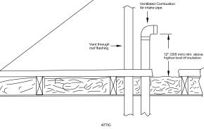
Fig. 48 – Vent Terminations for Ventilated Combustion Air A10497
