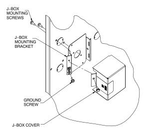
Fig. 35 – Installing J-Box (When Used)
