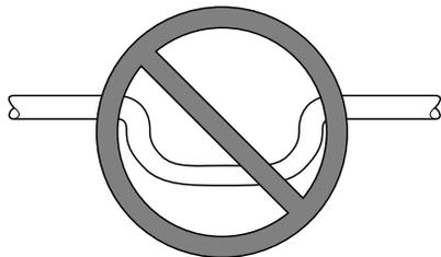
NE PAS UTILISER DE SIPHON CONSTITUÉ D'UN CONDUIT ÉTROIT!
