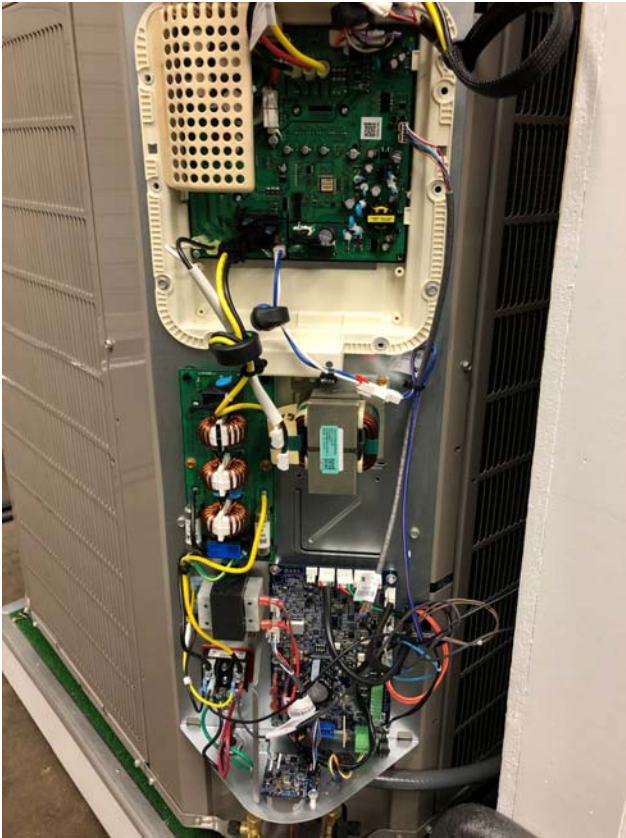
Fig. 19 – 2T/3T Control Box
