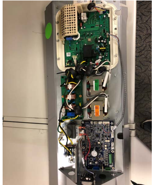
Fig. 20 – 4T/5T Control Box
