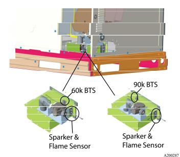
Fig. 20 – Burner Thermal Switch (BTS) (Ultra Low NOx) REMOVE SCREWS
