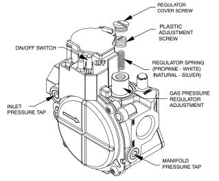
Fig. 13 - Standard Single-Stage Gas Valve
