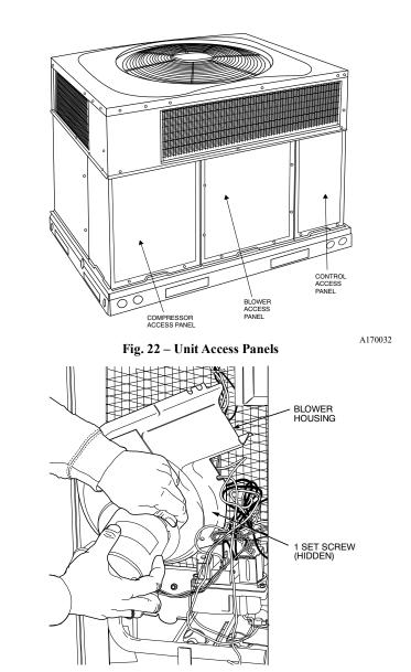
Fig. 23 – Removal of Motor and Blower Wheel
