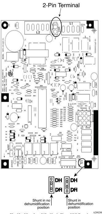
Fig. 19 - Ultra Low NOx Single Phase IGC Board
