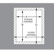
Fig. 11 – Floor and Plenum Opening Dimensions <u>Bottom Return Air Inlet</u> A96283
