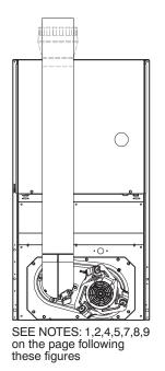
Fig. 33 – Downflow Application-Vent Elbow Up
