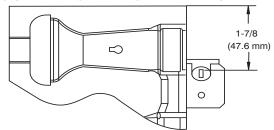
Fig. 48 – Igniter Position-Top View
