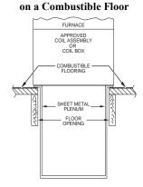
Fig. 12 – Furnace, Plenum, and Subbase Installed
