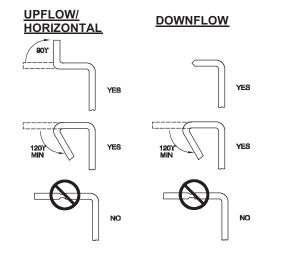
Fig. 17 – Duct Flanges
