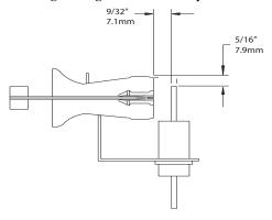
Fig. 49 – Igniter Position-Side View
