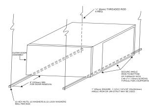
Fig. 15 - Horizontal Unit Suspension
