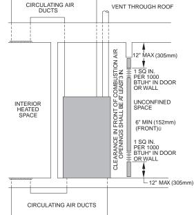
\*Minimum opening size is 100 in.2 with minimum dimensions of 3 in. (76 mm). \*Minimum of 3 in. (76 mm), when type -B1 vent is used.
