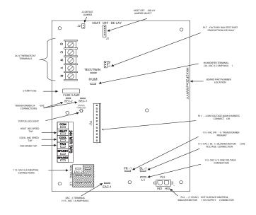
Fig. 28 – Furnace Control
