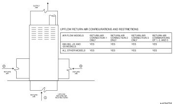
Fig. 19 – Upflow Return Air Configurations and Restrictions
