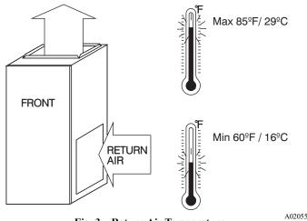
Fig. 3 – Return Air Temperature
