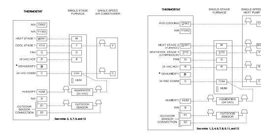
Single-Stage Furnace with Single-Speed Air Conditioner
