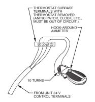
EXAMPLE: 5.0 AMPS ON AMMETER = 0.5 AMPS FOR THERMOSTAT ANTICIPATOR SETTING
