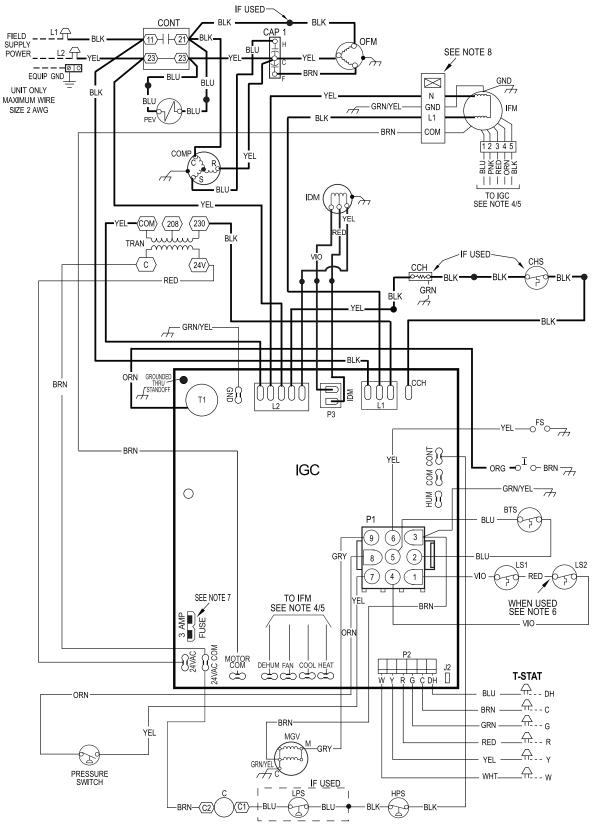
Fig. 15 – 208/230-1-60 Ultra Low NOx Connection Wiring Diagram
