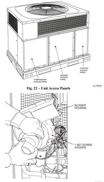
Fig. 23 - Removal of Motor and Blower Wheel
