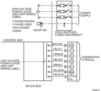
Fig. 10 – High- and Control-Voltage Connections
