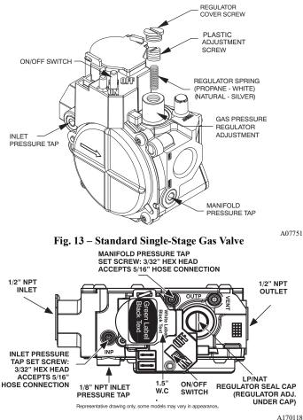
Fig. 14 – Single-Stage Gas Valve with Tower Pressure Ports
