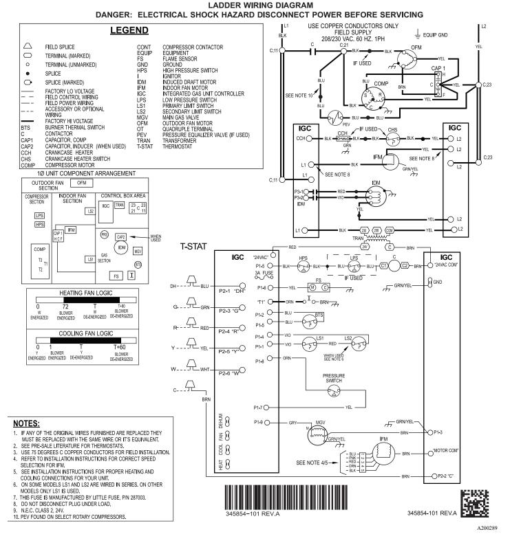
Fig. 16 – 208/230-1-60 Ultra Low NOx Ladder Wiring Diagram
